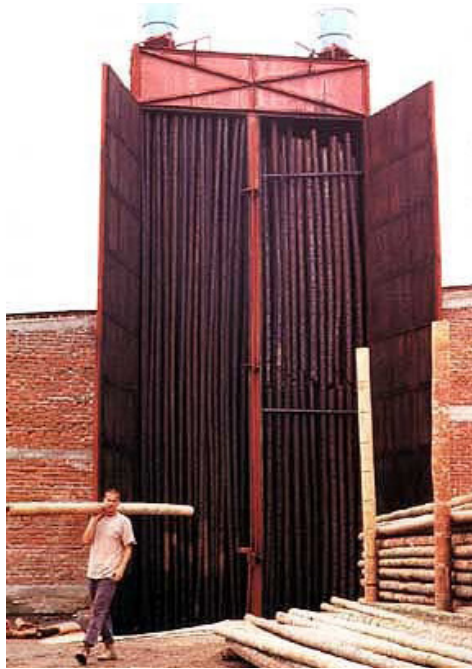
Figure 25 Smoking bamboo (N/A, 2015)
