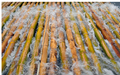
Figure 24 Leaching bamboo (N/A, 2012)
