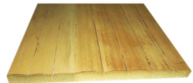
Figure 33 V-grooving result (Bakar et al., 2012, p. 177)
