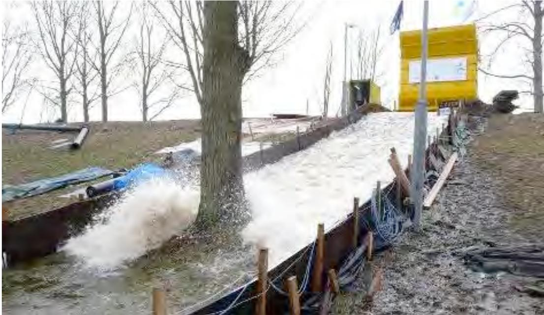
Figure 12-27 Overtopping Simulator (photo Infram)
