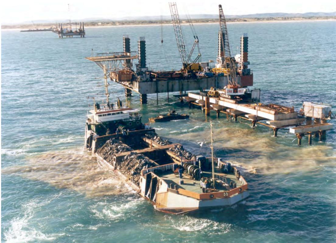
Figure 13-5 Side stone dumping vessel (Boskalis)
