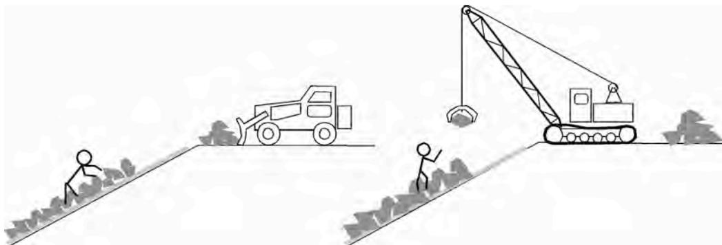
Figure 13-17 Placing of small and large stones from landside
