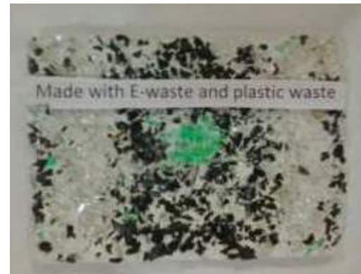
Figure 15: Tile made with waste from electrical and electronic equipment, waste from plastic and white cement. [32]
