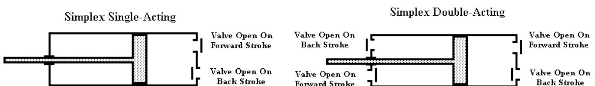
Figure 25: Single action linear displacement pump (left) and dual action linear displacement pump (right). Retrieved on 19-05-2015 from http://hawsepipe.net/chiefhelp/pumps/positive_displacment/reciprocating.htm
