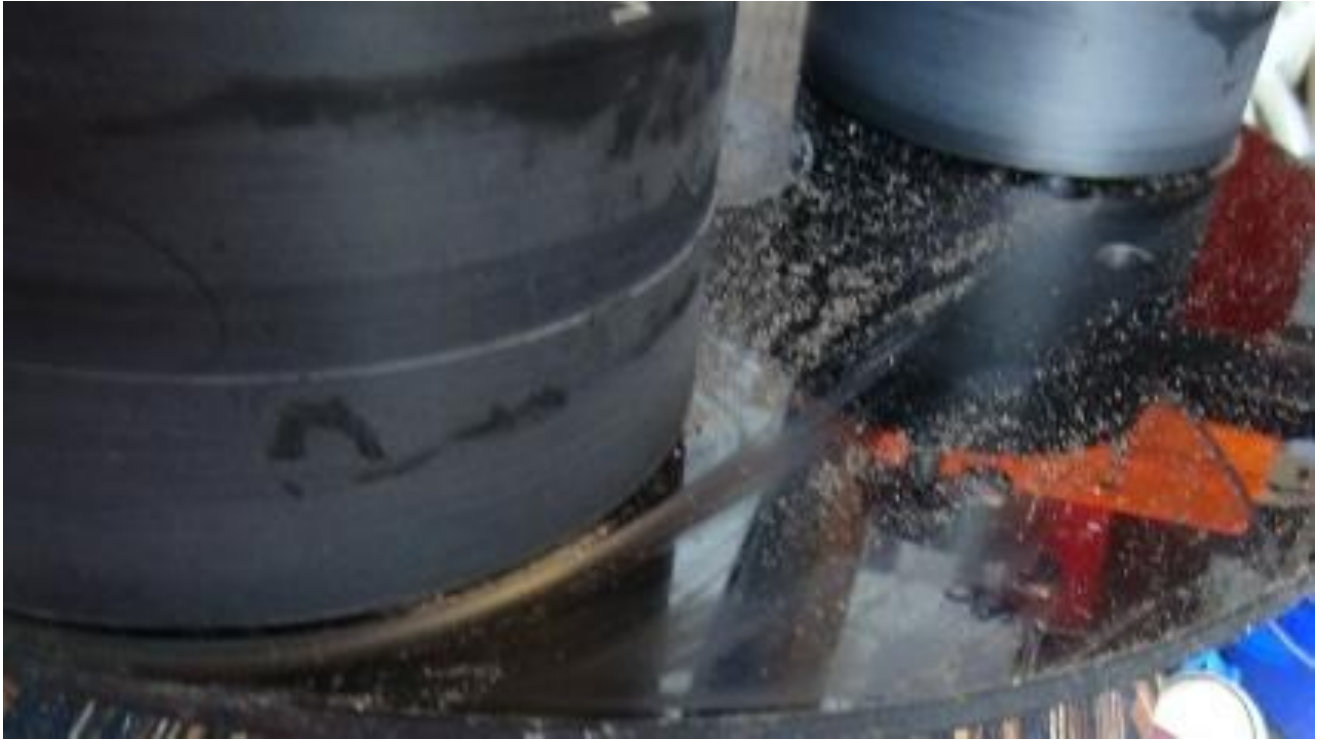
Figure 104: The rollers 'shave' into the impeller plates once their axis has released on one side.
