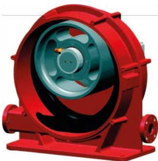
Figure 79: Peristaltic pump with a single roller. The hose passes by itself to avoid leakage. Retrieved on 14-7-2015 from http://empoweringpumps.com/water-scarcity-issues-may-solved-better-selection-pumping-technologies/
