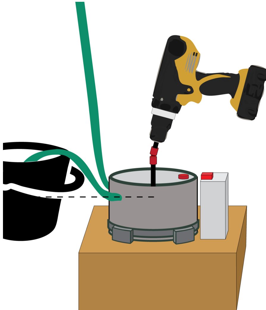
Figure 113 (right): Revised set-up, including cardanic coupling and fixation.
