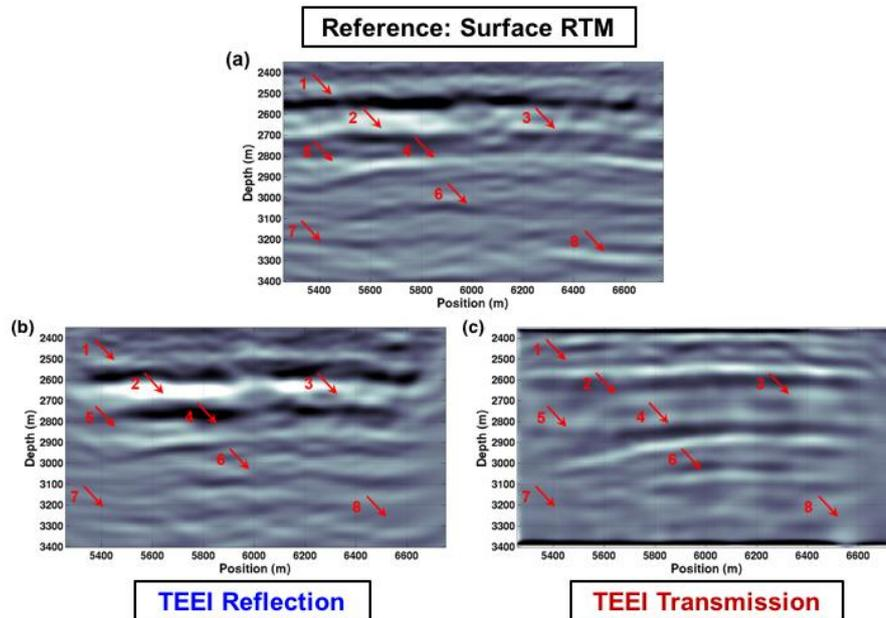
**Figure 4** Imaging of the structure within the target volume between the two chosen datums (**Figure 1**) from (a) conventional RTM of the surface reflection data, (b) local migration of the TEEI Reflection responses and (c) local imaging of the TEEI Transmission responses. The red arrows provide reference points for comparison between the images.
