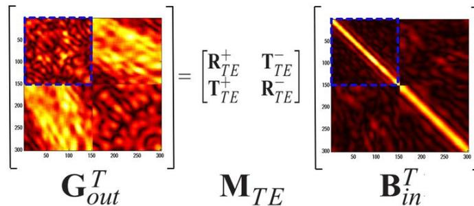
**Figure 2** Illustration of the full TEEI system in the form of normal equations, where the input  $\mathbf{G}_{out}$  is the desired  $\mathbf{M}_{TE}$  blurred by the operator  $\mathbf{B}_{in}$ . Here the coloured maps show the absolute values of the corresponding frequency-domain matrices from the field data example, for the datums as shown in Fig 1, at 40 Hz.
