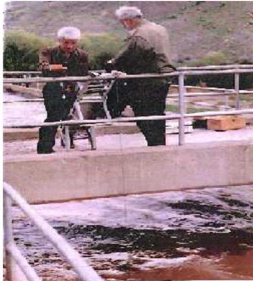
Figure. App 2.1. Water discharge measurements - current meter on Ziaran channel
