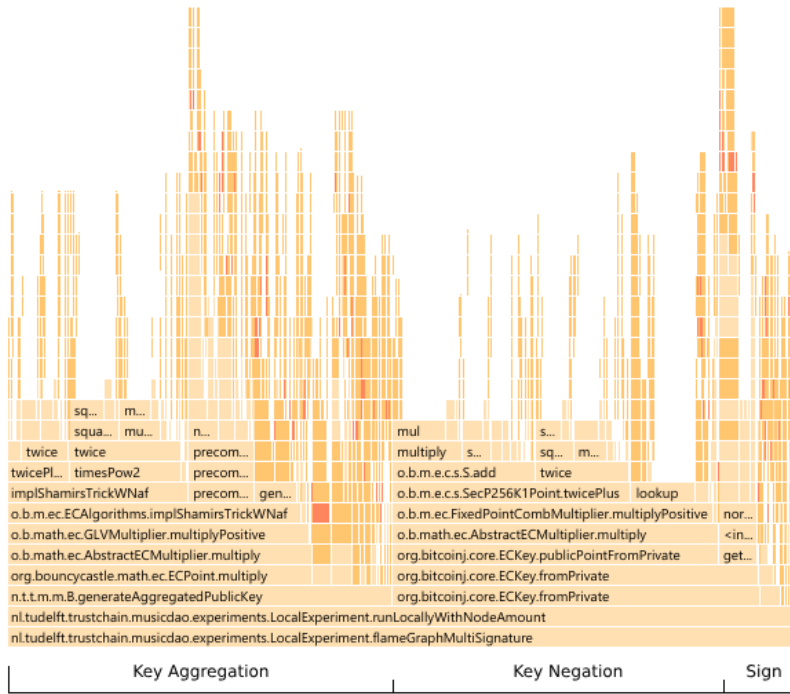
Fig. 8: Flame graph of the cryptographic operations in the governance protocol for 10.000 keys
