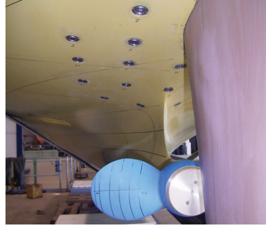
Figure 1: Two-bladed propeller fitted to the ship model equipped with flush-mounted pressure sensors
