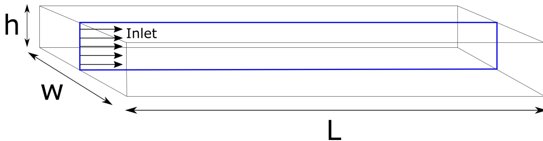
Figure 5.1: Illustration of the channel as it was modeled in ANSYS Fluent (blue). Not to scale.
