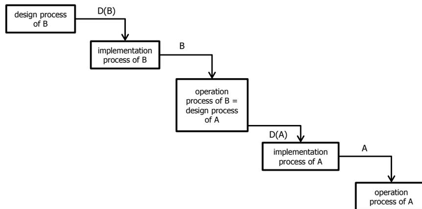
Fig. 4. Designing a design system (B) for the design of a system (A).
