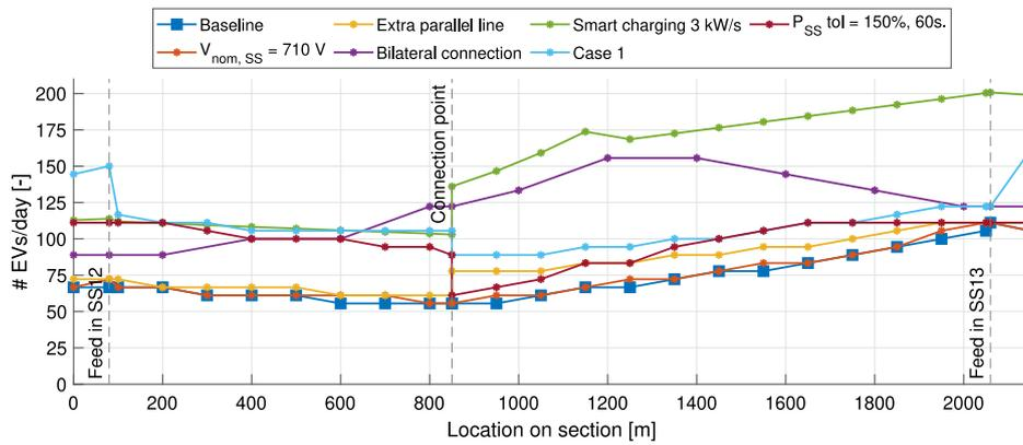
Fig. 15. Summary of various methods on the maximum achievable EV charging potential in supply zone A sections 23 and 2 on day 268. Case 1:  $V_{nom, SS} = 710$  V, an extra paralleled overhead line is added to the section, and the substation power rating is increased to 1100 kW.
