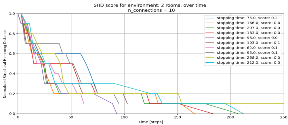
Figure 4.6: 10 runs of HBCD in the 2-room environment over with adjustment after each time step. Vertically is the normalized structural hamming distance.
