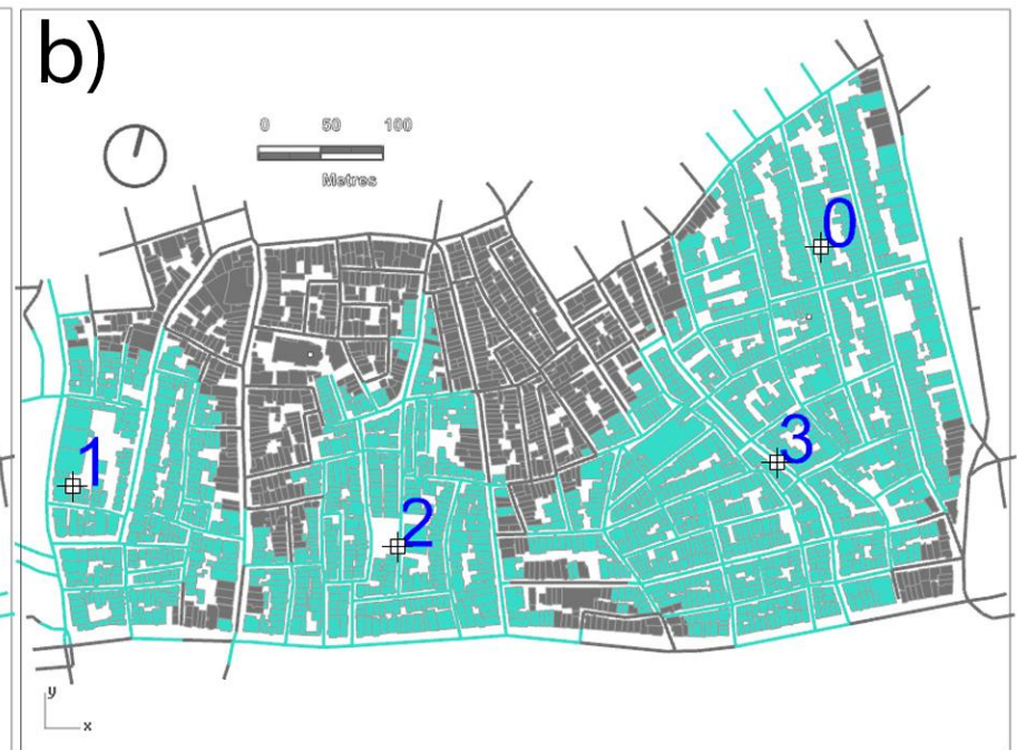
b) Vicinity catchment of POI (access to any POI), walking, considering the terrain when \tau=15
