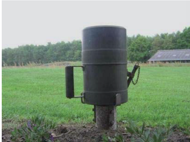
Figure 9-1 Manual rain gauge with a storage area of 2 dm 2 and an elevation of 40cm (top of bucket)
