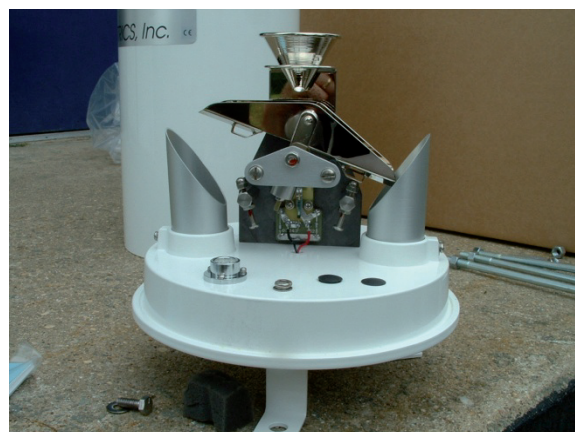
Figure 9-3 Tipping bucket rain gauge; every time the bucket tips over the actual time is registered. The surface area of the funnel and the volume of the bucket determine the precipitation unit of the tipping bucket.
