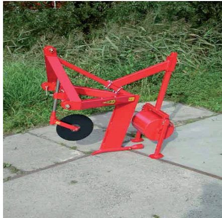
Figure 6-7 Mole plough which can be attached to a tractor. The disk in the front cuts through the grass and roots. The ball is ploughed through the ground after which the roll on the back of the frame closes the ground (source: www.wifo.nl ).
