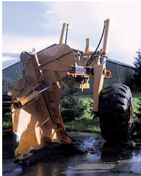
Figure 4-3 Trenching plough (ploughs up to 1.2 meters)
