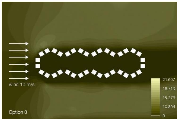
Fig 117: Option 0; Wind flow diagram of closed clusters.
