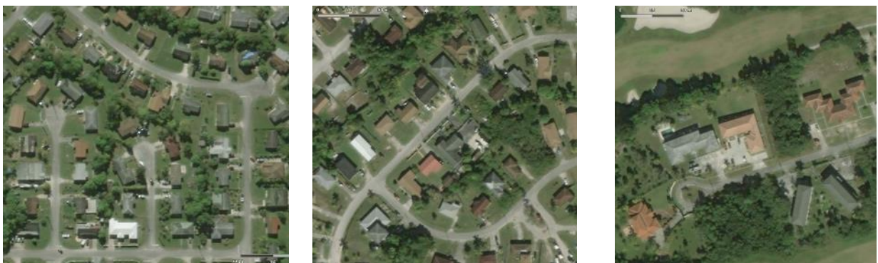
Fig 28: Visualization of existing densities in Grand Bahama, retrieved from Google Maps, from left: 15dw/ha, 11dw/ha, 4dw/ha.
