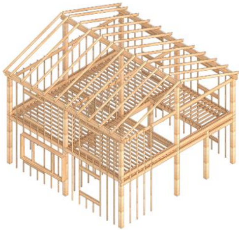
Fig 110: Wooden structure: a light wooden system to build the houses.
