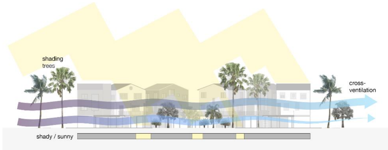
Fig 116: Courtyard cross-ventilation diagram.
