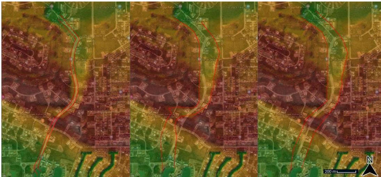
Fig 63: Placement boundaries of the wadi made with the program Hec-RAS: left "Following the road", middle "Following the natural elevation and width", right "Combination of following the road and following elevation".
