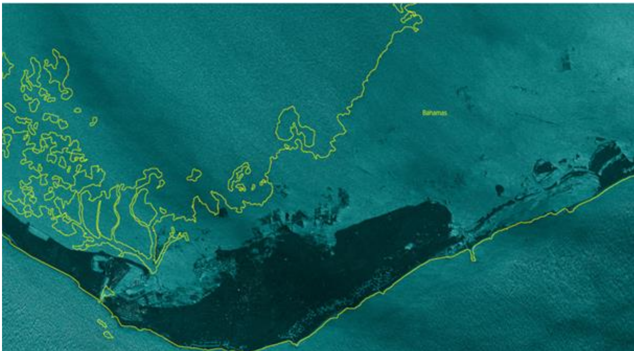
Fig 07: Grand Bahama Island during Hurricane Dorian. The image was taken 2 September 2019 and uses radar to penetrate the cloud cover. Areas that appear nearly black are not flooded (ICEYE, 2019).
