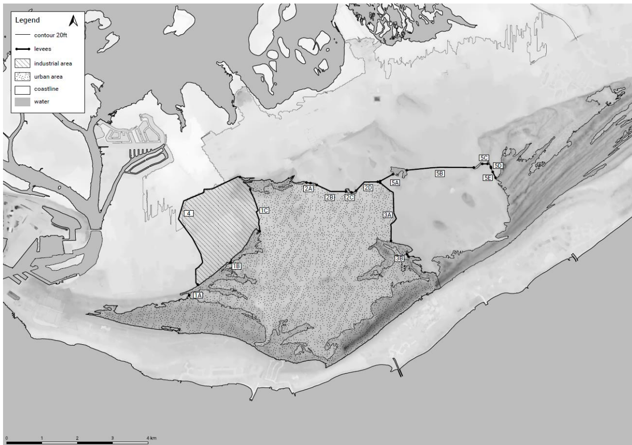
Fig 49: Levees with their corresponding number and the 20 feet contours, surrounding the proposed collective protected area of Freeport which is divided in the industrial and urban area.
