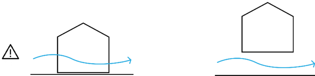
Fig 102: Concept diagram: lifting the houses.
