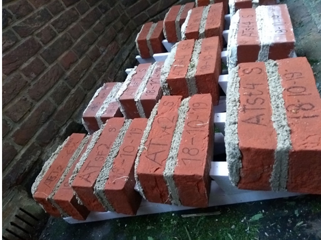
Fig. 3. Brick-mortar specimens in outdoor conditions.
