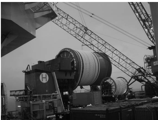
Figure 10: Capstan drum on a ship of Heerema.
