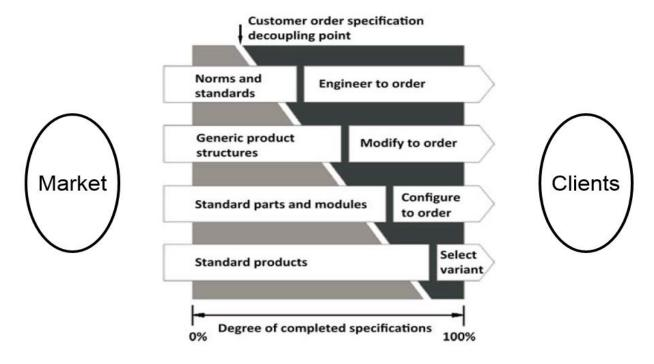
Figure 7 CODP in different supply chain structures modified from Segerstedt and Olofsson (2010)
