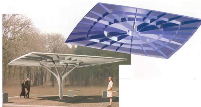
Fig.Ap3. 24. The roof of the shed is 25mm thick and the stiffening ribs are 40mm thick
