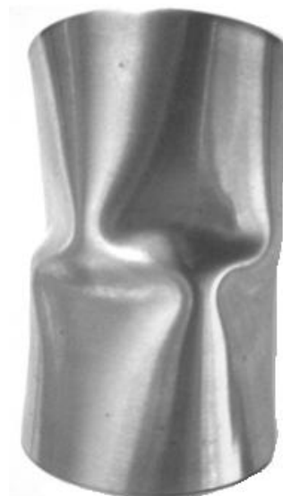
Fig.B25. Experiment on an aluminum hyperboloid toothbrush holder (Yoshimura pattern) [RtM]
