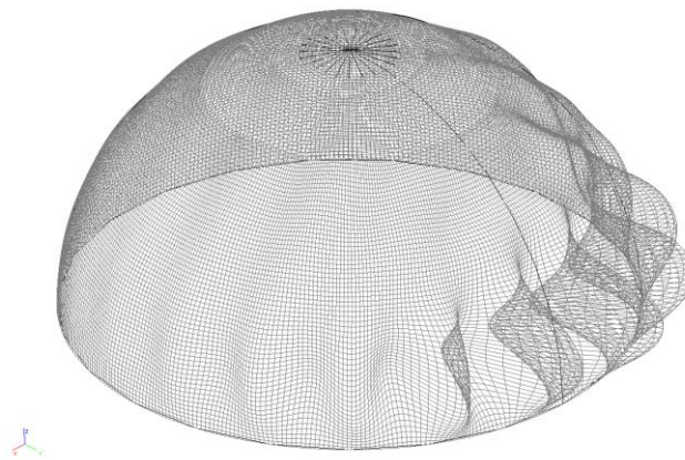
Fig.App5.2. First buckling pattern for load case 2
