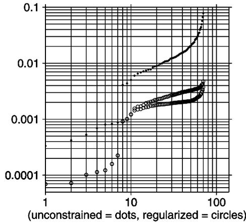
**Figure 1.** Square root of eigenvalues of the inverse normal matrix, unconstrained (dots) and regularized (circles, for the two damping parameter used in the real-data analysis) inversion, in m. Inversion for degree-7 expansion and Helmert parameters.
