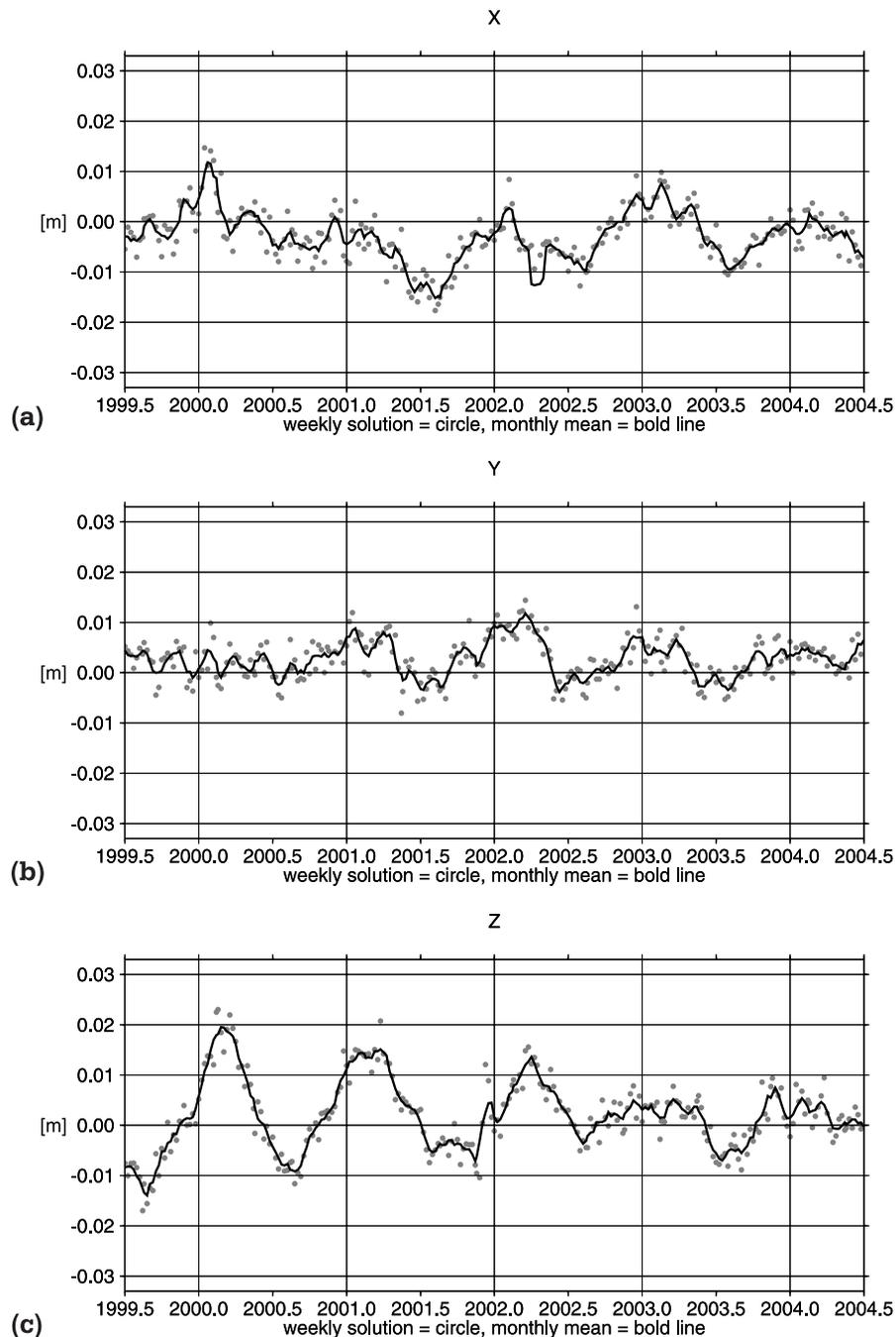
**Figure 2.** Load moment expressed as CF frame variation [m] with respect to CM from GPS inversion, in X, Y, Z direction (CF center of figure system, CM joint center of mass of Earth and load). Weekly estimates (dots), and running 30 day mean (line).
