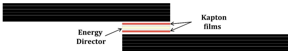
Figure 3.6. Schematic of specimen prepared for removing the energy directors from the weldline in order to perform direct crystallinity measurements. Dimensions are not to scale.
