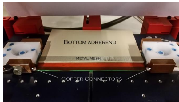
Figure 2.2. Preparation of RW joints. The metal mesh is placed over the bottom adherend while being in good contact with the copper connectors in order to ensure electrical current circulation.
