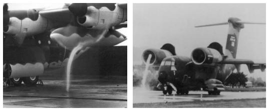
(a) Ground vortices toward the propeller of C130 aircraft<sup>[1]</sup>
