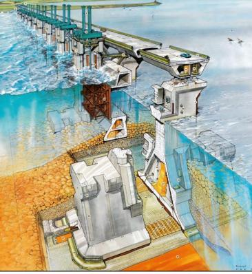
Figure A.26: Overview of the components of the OSK (Steeneporte, 2014).
