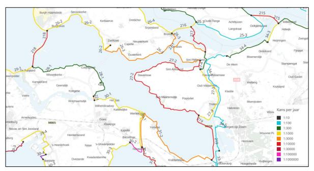
Figure A.39: Safety standards for flood defences in the Eastern Scheldt estuary (Rijkswaterstaat, 2017e).
