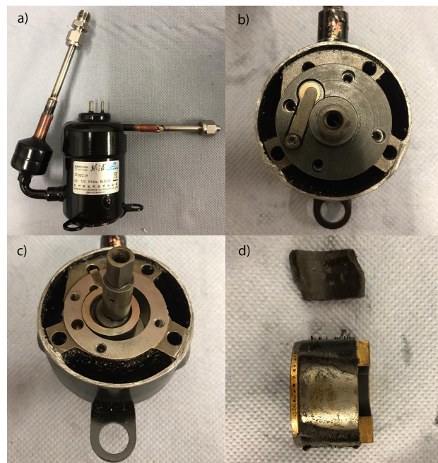
Fig. 2. a) Purswave 1.9 cc rolling piston compressor. b) Compressor internals including discharge reed valve. c) Compressor internals including crankshaft, rolling piston and vane. d) Rotor failure due to overheating.
