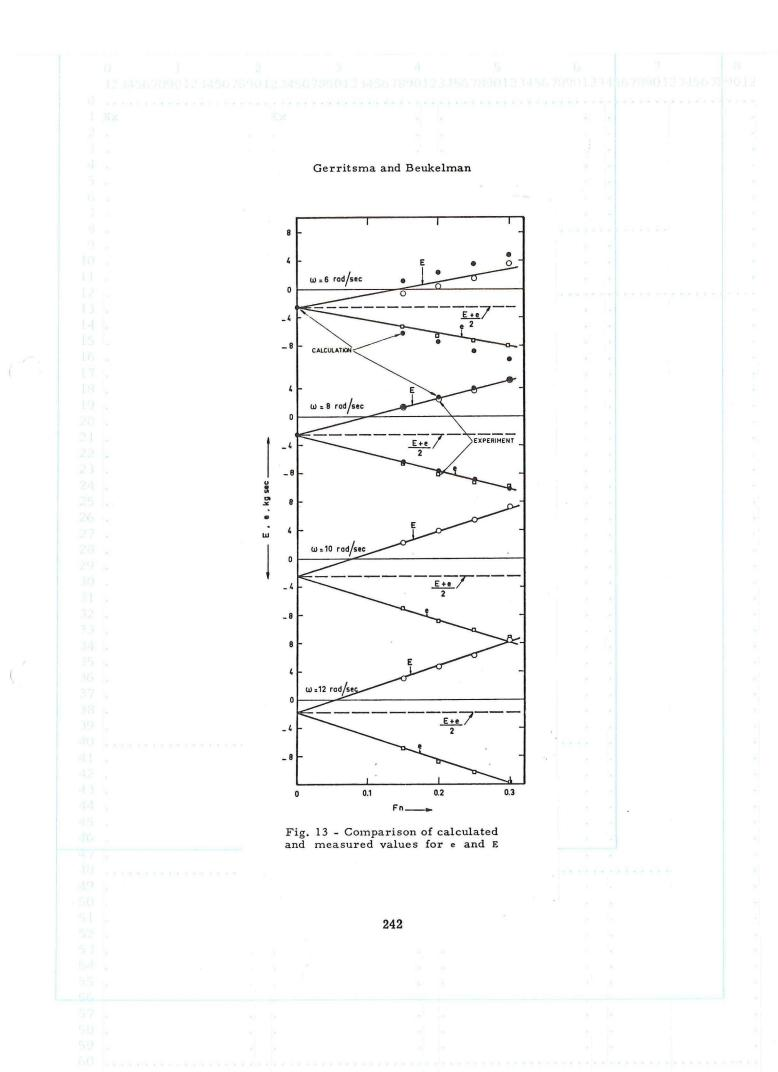
The calculated values are in line with the experimental results. The natural frequencies for pitch and heave are respectively  $\omega = 7.0/6.9$  rad/sec and in this important region the calculation of the damping cross-coupling coefficients is quite satisfactory. The zero speed case will be studied in the near future by oscillating experiments in a wide basin to avoid wall influence.
