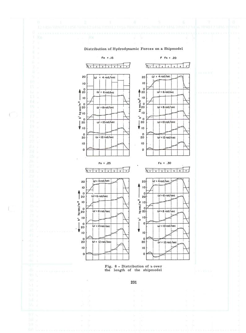
In Fig. 8 it is shown that the distribution of the damping coefficient b depends on forward speed and frequency of oscillation. The damping coefficient of the forward part of the shipmodel increases when the speed is increasing. At the same time a decrease of the damping coefficient of the afterbody is noticed. For high frequencies negative values for the cross-sectional damping coefficients are found.
