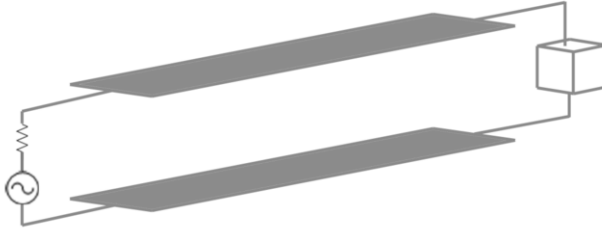
Figure 1: Geometrical structure of a parallel plate waveguide used to verify the proposed algorithm.
