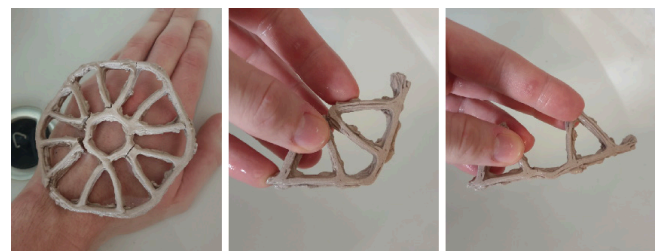
Fig. 73. Flexibility fail & flexibility proof
