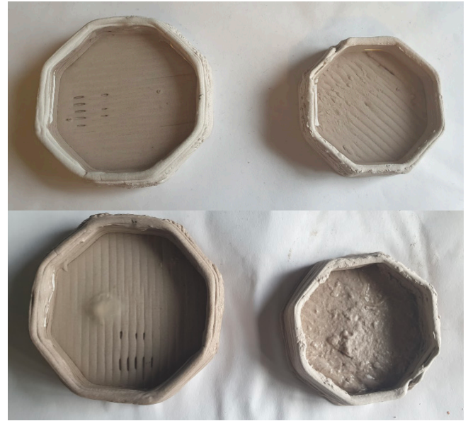
Fig. 80. Effect of water on cross-linked and non-cross-linked prints.
