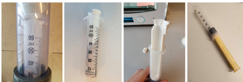
Fig. 34a,b,c,d. System can not print the viscous paste
