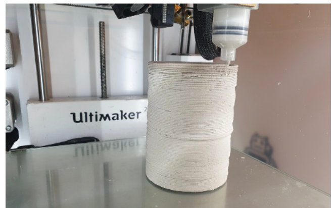
Fig. 42. 100mm tall object printed with new setup
