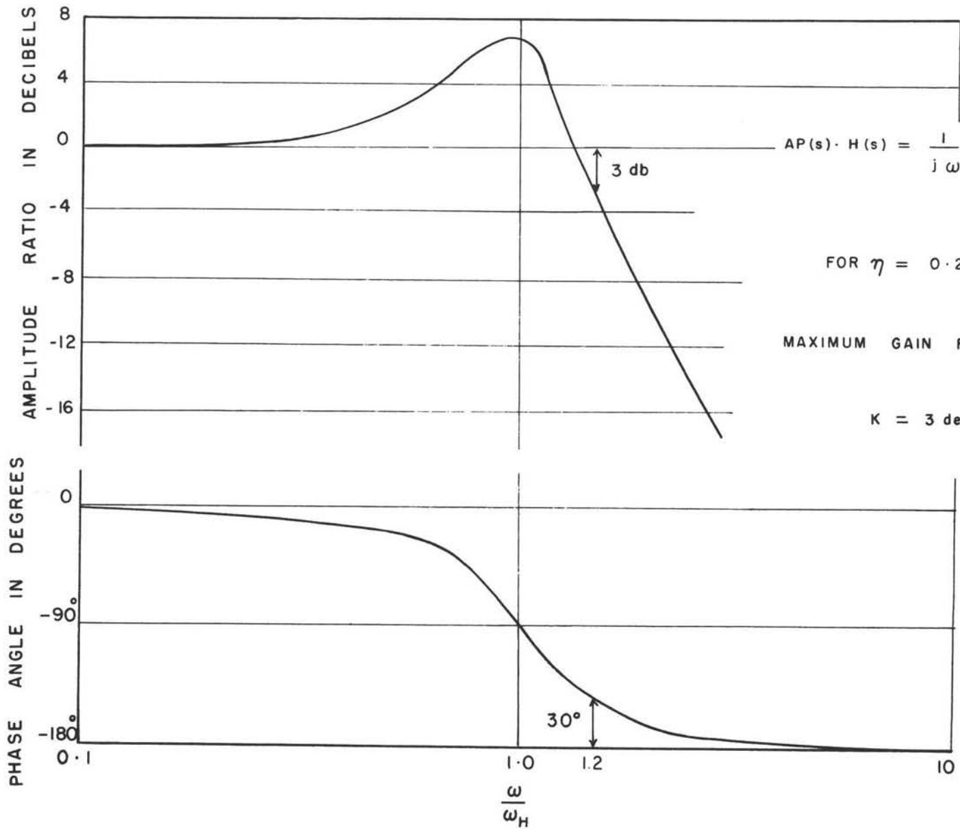
$$AP(s) \cdot H(s) = \frac{1}{j\omega} \times \frac{j\omega}{\left[ \left( \frac{\omega}{\omega_H} \right)^2 + 2\eta j \frac{\omega}{\omega_H} + 1 \right]}$$
