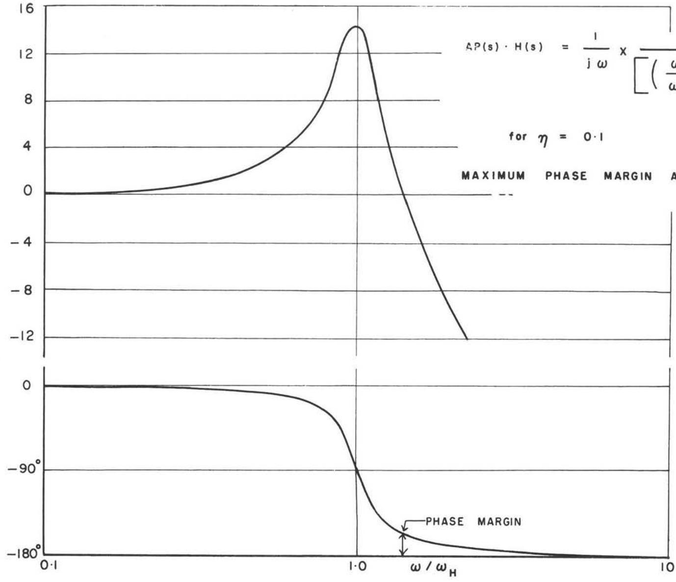
$$AP(s) \cdot H(s) = \frac{1}{j\omega} \times \frac{j\omega}{\left[ \left( \frac{\omega}{\omega_H} \right)^2 + 2\eta \left( \frac{\omega}{\omega_H} \right) + 1 \right]}$$
