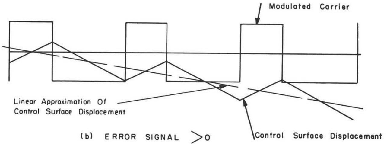
LINEARIZATION OF "BANG-BANG" SERVO ACTUATOR
