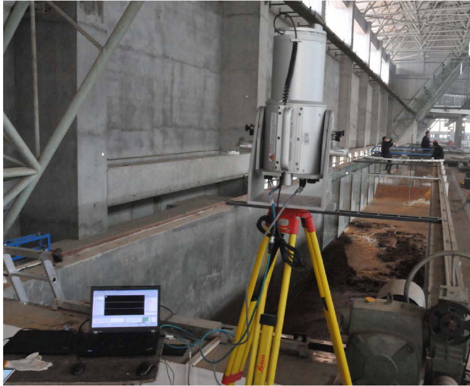
Figure 19 Three Dimensional Laser Scanner Systems
