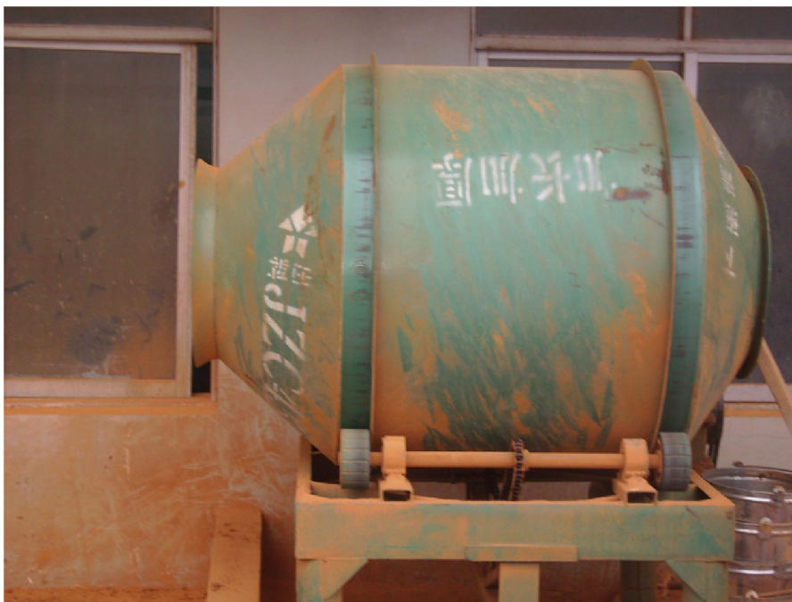
Figure 25 Blender to reproduce the soil sample
