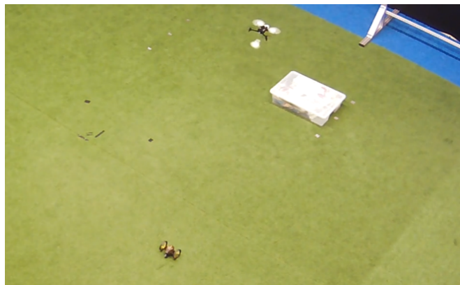
Fig. 14. The UAV carries and drops the tennis ball where the elevation of the terrain should be estimated. The UGV positions itself in an adequate perspective to estimate the elevation.
