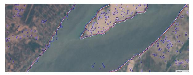
Figure 5.56: Close-up of RGB image in the region of Katha with the edges calculated with the threshold values in table 5.4 for the NDWI (red), MNDWI (white) and backscatter (blue).
