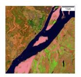
Figure 5.15: False color composite, made with the 'swir', 'nir' and 'green' bands of the Sentinel-2 image covering the Katha polygon on 07-03-2018.
