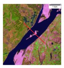
Figure 5.31: False color composite of Katha, made with the 'swir', 'nir' and 'green' bands of the Sentinel-2 satellite covering the Katha region when the river is wide and no bar is visible on 07-11-2017.
