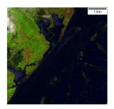
Figure 5.18: False color composite, made with the 'swir', 'nir' and 'green' bands of the Sentinel-2 image covering the Katha polygon on 19-08-2017.
