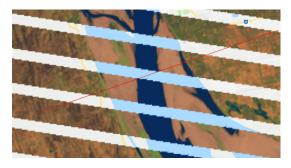
Figure 2.9: Cross-section at the Magway station at 14-03-2007. Due to failure of the Landsat 7 mission part of the river cross-section is not taken into account.
