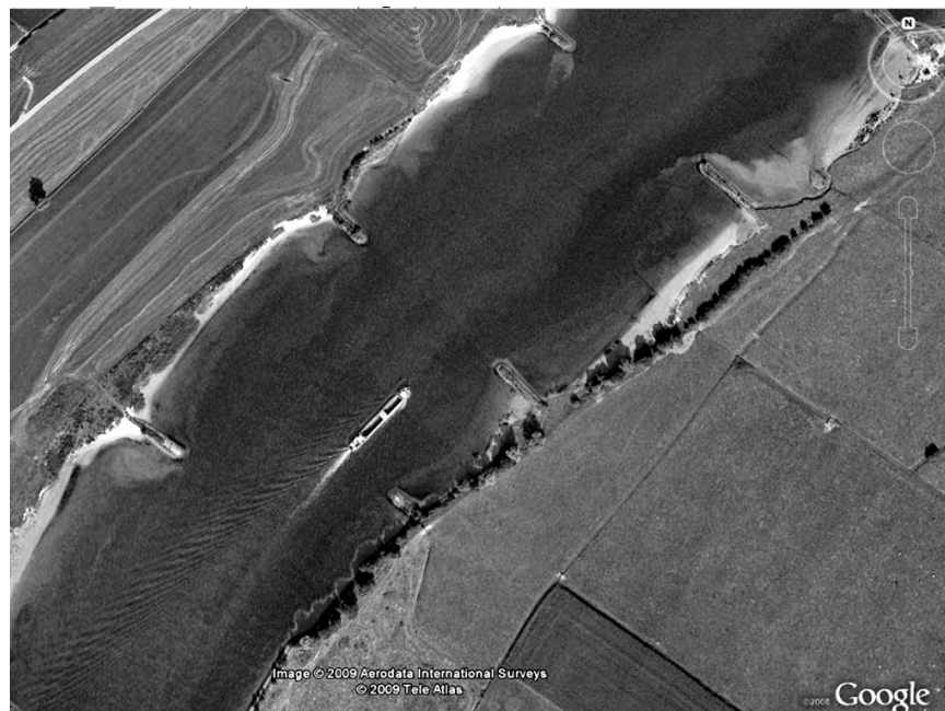
Figure 1.5: Separating and recirculating flow in groyne fields along the river Lek, Vianen, Netherlands (source: Google Earth 2010).
