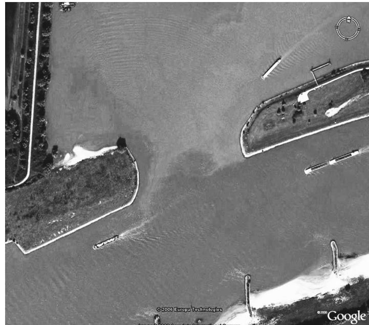
Figure 1.4: Large eddies due to flow separation at a harbor entrance along the river Waal, Ochten, Netherlands (source: Google Earth 2010).
