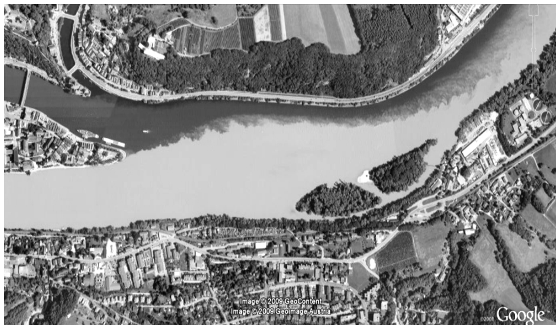
Figure 1.3: Shallow mixing layer at the confluence of the rivers Danube and Inn, Passau, Germany (source: Google Earth 2010).
