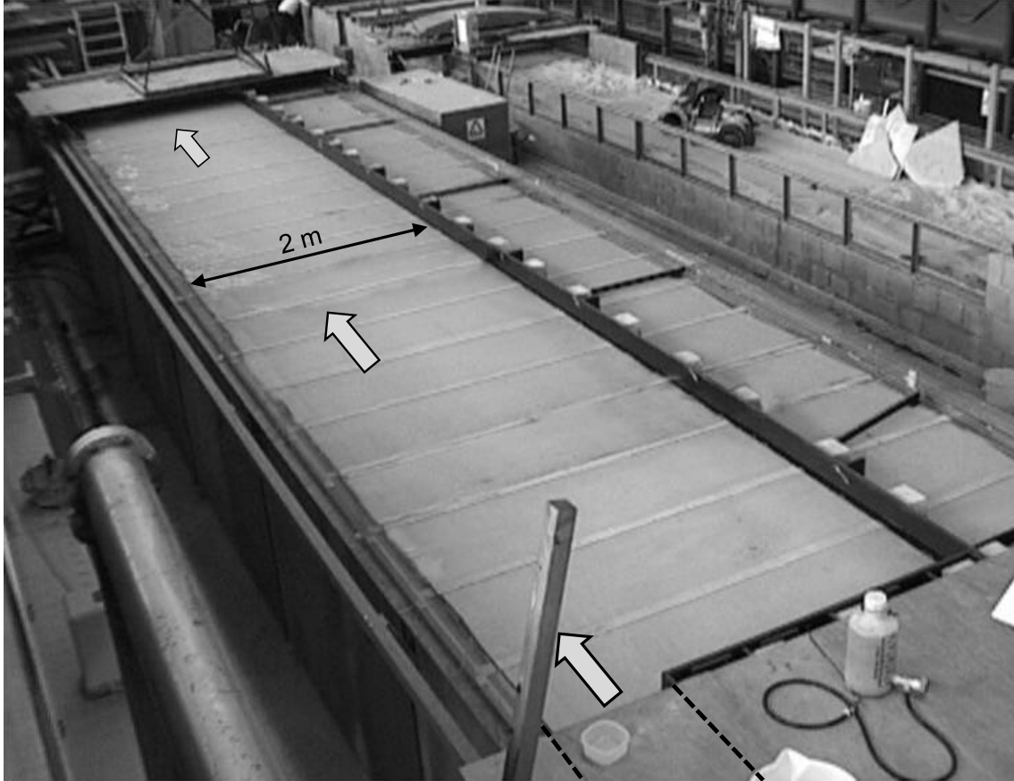
Figure 3.3: Picture of the experimental SLE setup; flume width and main flow direction have been indicated. The background shows part of the movable bridge construction on which the digital camera has been placed.
