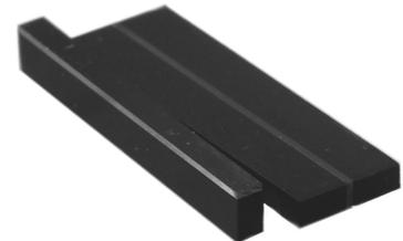
Figure 4.18: Specimen delaminated from its neighbor during dicing.
