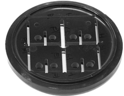
Figure 4.13: Four CT specimens milled from an EMC plate. One CT specimen is 25 mm wide. The dimensions followed the geometry defined by Walter 2003.
