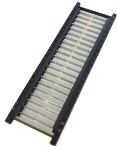
Figure 4.9: Assembly of silicon strips placed between two bearings. Here shown for a gold release layer at the center of each strip, for 4PB use.
