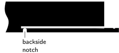
Figure 4.3: A notch below the interface decouples the load lip from the clamping body.
