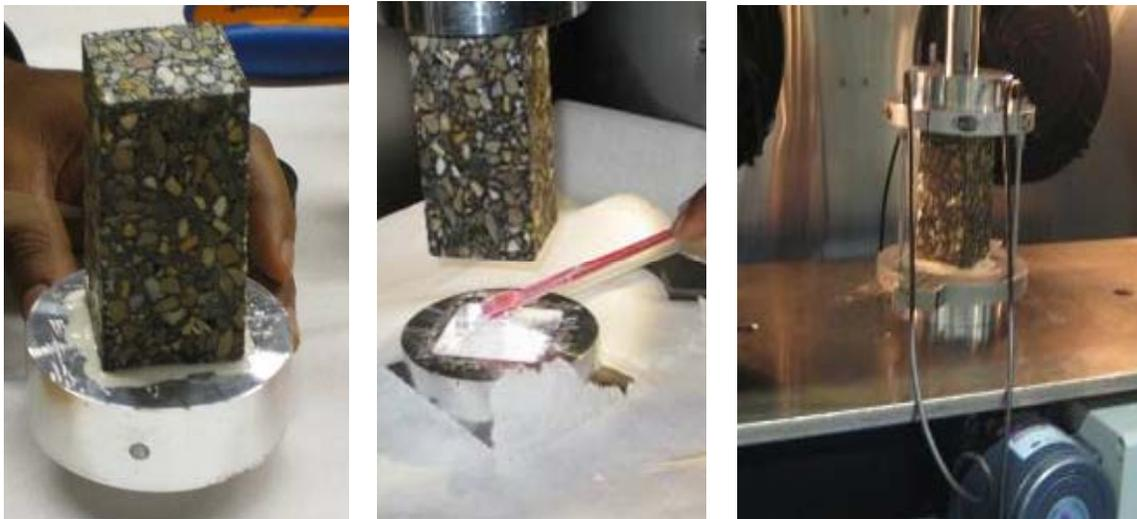
Fig.3 Uni-axial setup: mounting procedures (left and middle), strain transducers (right)
