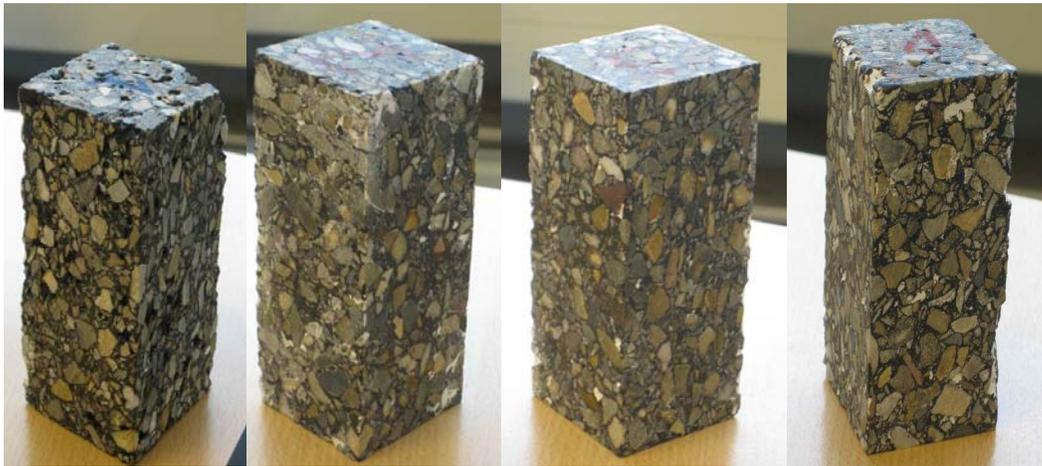
Fig. 2 AC mixture specimens
