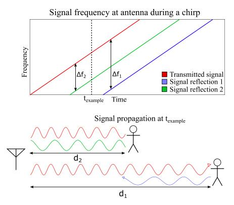
Figure 2.2: A FMCW radar uses a chirp of increasing frequency to determine the range to a target. Due to the signal travel time, The frequency of the transmitted signal and received reflection will be shifted by an amount linearly related to the distance of the object.
