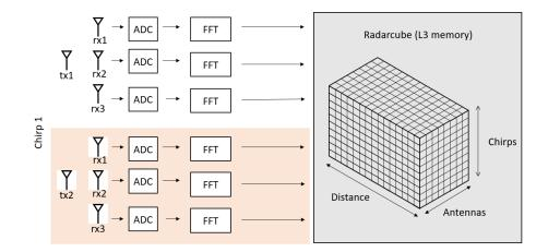
Figure 2.4: Capturing a chirp on a system with 2 TX and 3 RX antennas. The two TX (Transmitter) antennas chirp after eachother. Every RX (Receiver) antenna receives the chirp simultaneously. The DSP performs a range FFT whose results are stored in the radar cube before the next chirp. The angle of arrival and object velocities can be calculated by performing an FFT in the antennas and chirp dimensions respectively.
