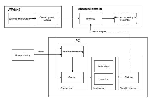
Figure 3.3: A schematic overview of the test setup.
