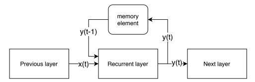
Figure 4.11: Basic structure of a recurrent layer. The output of the previous time step is fed back into the same layer in the current time step.
