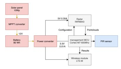
Figure 3.5: Schematic design of the inference system that can be deployed at playgrounds.
