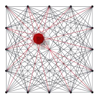
Figure 2.1: Operating principle of Radio Tomographic Imaging. Every node measures the RSS of radio transmissions from every other node. Radio links that are obstructed by an object in its fresnel zone (in red) have a reduced RSS. By using a model of the radio channel, the locations of obstructions can be estimated. In this example, we use the average signal strength of all links passing over a pixel to color it.
