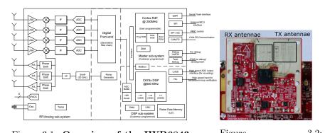
Figure 3.1: Overview of the IWR6843 com-Figure ponents [53]. IWR6
