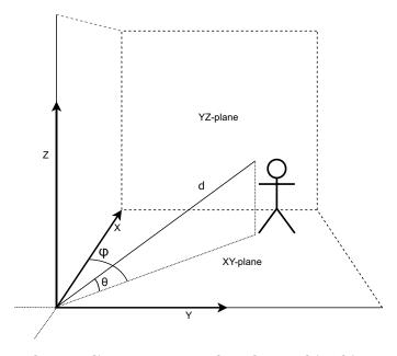
Figure 1.2: The coordinate system and angles used in this report. We always use the reference frame of the sensor, unless specified otherwise. A location in the coordinate system can be defined by both the carthesian coordinates (xyz), or by the polar coordinates of distance (d), Azimuth  $(\Phi)$  and Elevation  $(\theta)$ .
