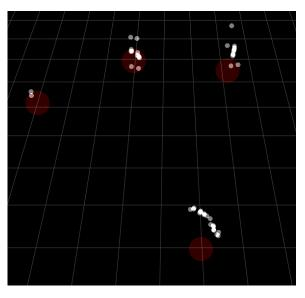
Figure 4.2: Point clouds of four children playing. The grid size is 1 meter. Brightness represents signal strength, velocity is not shown.
