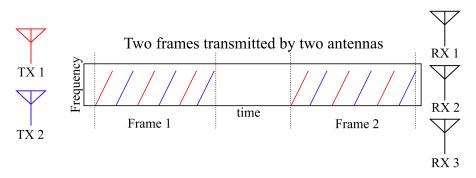
Figure 2.3: The radar transmits multiple chirps in a frame. Multiple frames follow each other after a delay. The chirps are transmitted from multiple antennas and received by multiple antennas.
