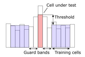
Figure 2.5: CA-CFAR peak detector. The value of the cell under test is compared to the average value of the training cells plus a threshold value. Guard bands are excluded from the training cells to avoid the sidelobes of the peak from affecting the average. The number of training cells, guard bands and the height of the threshold can be modified.
