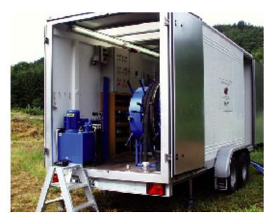
The flow rate is 1 m<sup>3</sup>/h and the efficiency for capture of particles > 0.45  $\mu$ m is about 90 %, as tested with filters. An amount of about 400 g SPM is sampled in one run.
