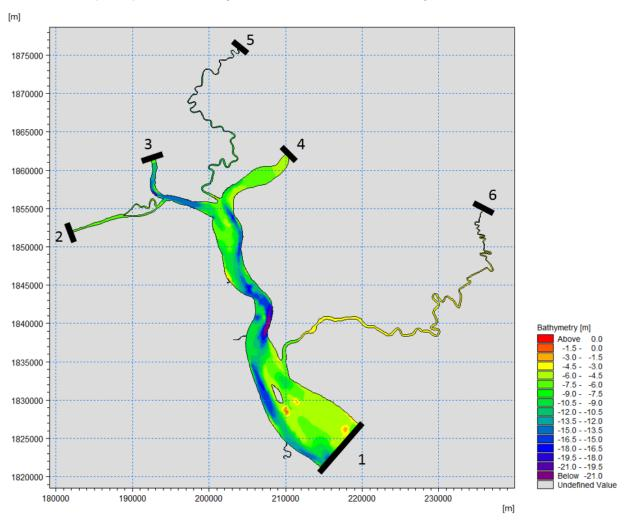
Figure 5.1: Model domain with boundary conditions. 1: Water level time-series. 2: Discharge time-series Twante Canal. 3: Discharge time-series Hlaing River. 4: Discharge time-series Bago River. 5: Land boundary. 6: Land boundary
