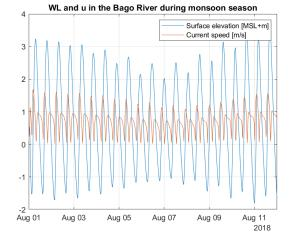
Figure 5.26: Surface elevation (WL) and current speed (u) in the Bago River during monsoon season
