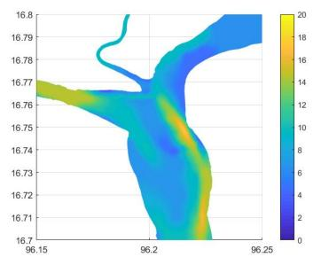
Figure 8.1: Bathymetry after deepening of Monkey Point Channel in m below MSL
