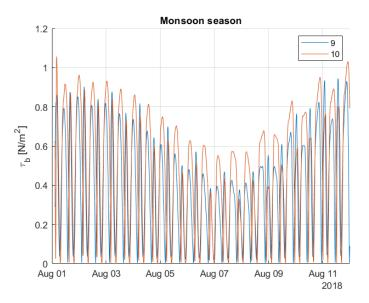
Figure 6.13: Bed shear stress on the northern shoal (9) and southern shoal (10) during the monsoon season. The maximum shear stress occur during spring tide and the minimum shear stresses occur during neap tide.
