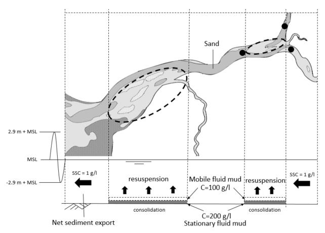
Figure 7.3: Conceptual diagram for the SSC during spring tidal conditions in the monsoon season
