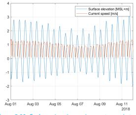
Figure 5.22: Surface elevation and current speed at location 7 during monsoon season
