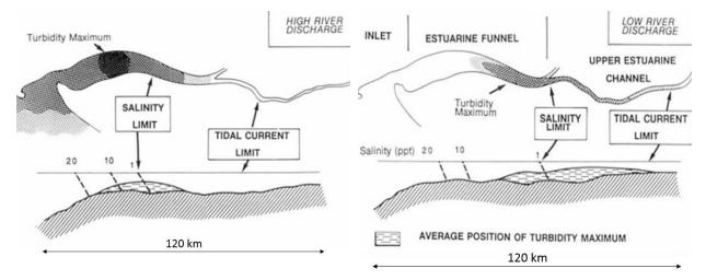
Figure 4.2: Location of the ETM in the Gironde Estuary for high and low river discharge. Source: (Allen G., 1991)
