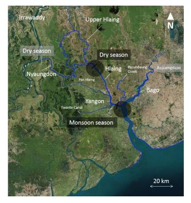
Figure 4.4: Potential locations of ETM based on the salt intrusion. The black circles indicate the potential ETM location per season.
