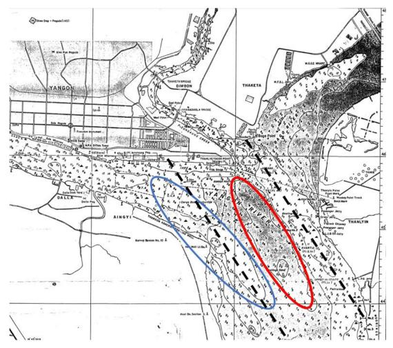
Figure 2.18: Nautical chart 2007; zoom Inner Bar. The blue oval represents the channel evolution. The red oval highlights the Hoasting's shoal. The black dashed lines indicate the parallel channels of the Bago River and Yangon River
