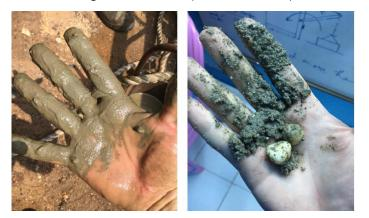
Figure 2.7: Dredged sediment by Boskalis (2016). Left: Very soft clayey fine sand from the middle of the channel. Right: medium sand with gravel from the south slope (Inner Bar)
