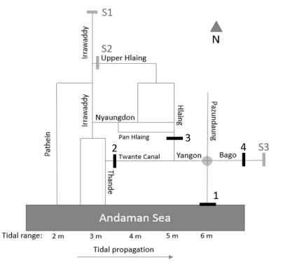
Figure 5.2: Output locations of discharge time series in SOBEK model. S1: Discharge time-series of Irrawaddy River. S2: Discharge time-series of Upper Hlaing River. S3: Discharge time-series of Bago River. 1: Water level time-series. 2+3+4: Output locations in SOBEK for discharge time-series as boundary conditions in MIKE.
