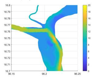
Figure 8.4: Bathymetry after increasing the dimensions of Monkey Point Channel in m below MSL
