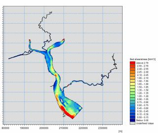
Figure 6.4: Maximum bed shear stress during spring flood in dry season
