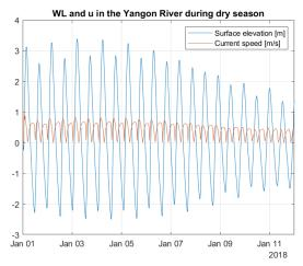
Figure 5.27: Surface elevation (WL) and current speed (u) in the Yangon River during dry season
