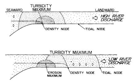
Figure 4.1: Conceptual diagram showing the seasonal displacement of an estuary turbidity maximum. Density processes dominate the trapping of fine sediment during high river discharge, tidal processes dominate during low river discharge. The density node represents the salt intrusion limit and the tidal node represents the tidal intrusion limit. Source: (Wells, 1995)
