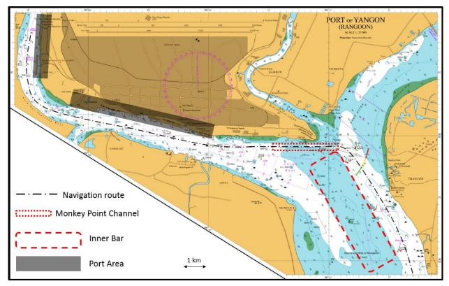
Figure 2.2: Bathymetry of he confluence of the Bago River and the Yangon River with the navigation channel highlighted by the dashed line. Source: (RHDHV, 2016)
