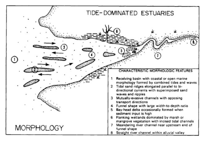
Figure 3.2: Characteristic morphologic features of a tide-dominated estuary (Wells, 1995)
