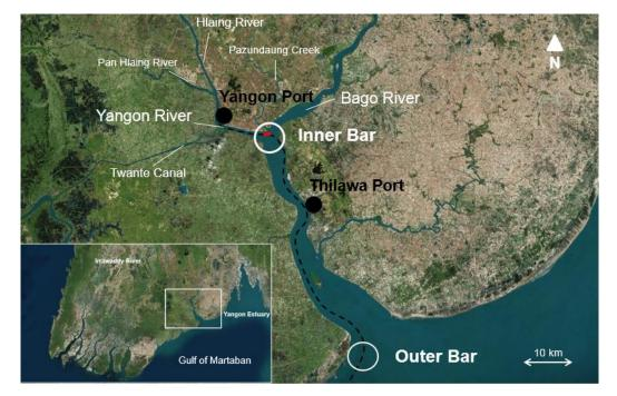
Figure 1.2: Yangon Estuary with the Inner Bar and Outer Bar. The black dashed line shows the navigation channel. The red line shows the location of Monkey Point Channel.
