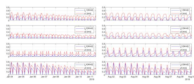
Figure 6.15: Bed shear stress and current velocity in locations 1,2,3 and 4 during spring and neap tide in dry season
