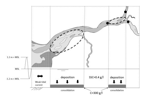
Figure 4.5: Conceptual diagram of deposition and consolidation of fine sediments on the shoals during neap tide. The black dots represent the locations where the SSC is measured.
