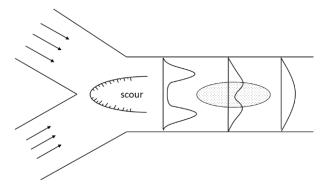
Figure 4.8: Principle of mid-channel bar growth (Ashworth, 1996)
