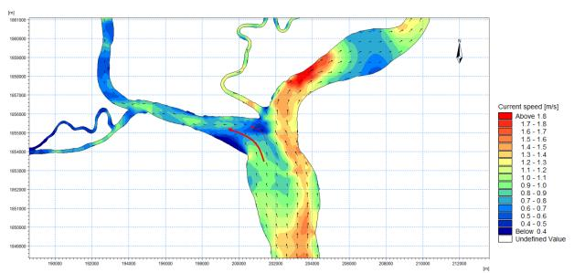
Figure 8.9: Flow velocities with direction during spring tide in dry season. The large red arrow indicates the dominant flow and the smaller red arrow indicates the minor flow.
