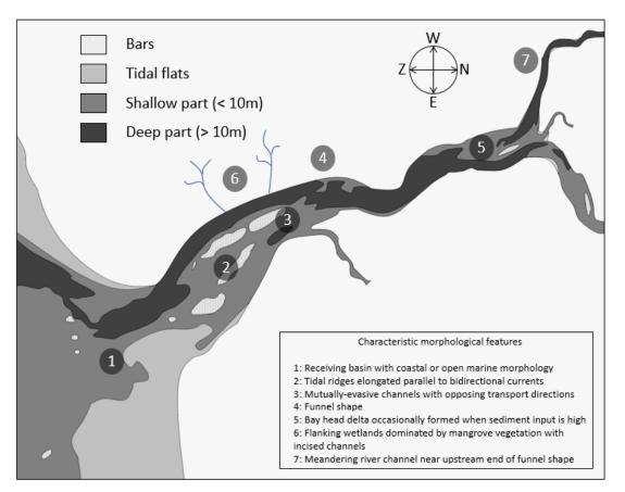
Figure 3.3: Characteristic morphologic features of the Yangon Estuary
