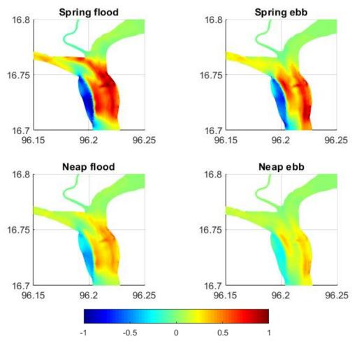
Figure 8.14: Increase in bed shear stress [N/m<sup>2</sup>] after construction of the adjustment at the western bank
