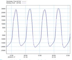
Figure 13.14: Comparison of discharge downstream of the confluence of the Bago and Yangon rivers
