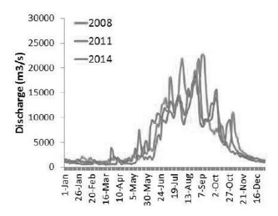
Figure 2.3: Measured discharge of the Irrawaddy River (DMH, 2014).
