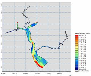
Figure 6.8: Maximum bed shear stress during spring flood in monsoon season
