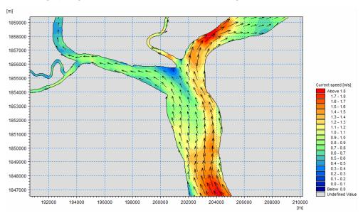
Figure 5.33: Current speed during spring flood in dry season
