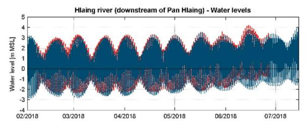
Figure 13.9: Simulated (blue) versus measured (red) water level on Hliang River (station KIP) from February until July 2018
