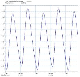
Figure 13.13: Comparison of the water level downstream of the confluence of the Bago and Yangon Rivers
