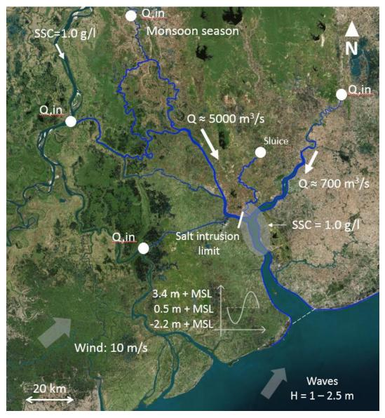
Figure 2.20: Stage 1 conceptual model, monsoon season. Q,in is the symbol for the locations where water enters the system. Q is the average discharge. SSC Is the measured suspended sediment concentration within the oval. H is the wave height.
