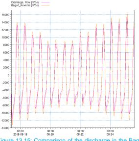
Figure 13.15: Comparison of the discharge in the Bago River
