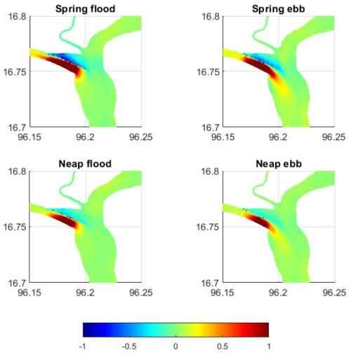
Figure 8.13: Increase in bed shear stress [N/m2] after construction of the adjustment at the split
