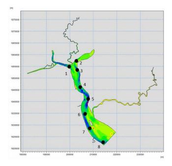
Figure 5.20: Locations to calculate the water levels and current speeds along the estuary
