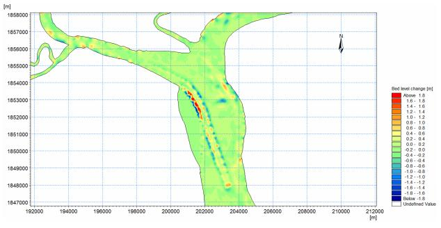
Figure 8.18: Morphodynamic response after one month of sand transport
