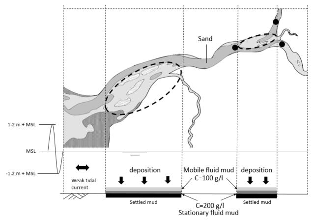
Figure 7.1: Conceptual diagram for the SSC during neap tidal conditions for both the dry season and monsoon season
