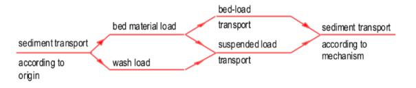
Figure 4.12: Types of sediment transport (Blom, 2016)
