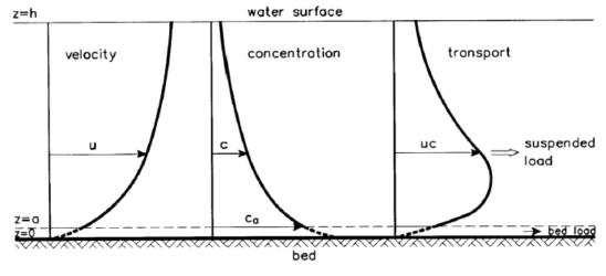
Figure 4.13: Distinction between bed-load transport and suspended-load transport by means of a reference height z=a (Van Rijn, 2003)
