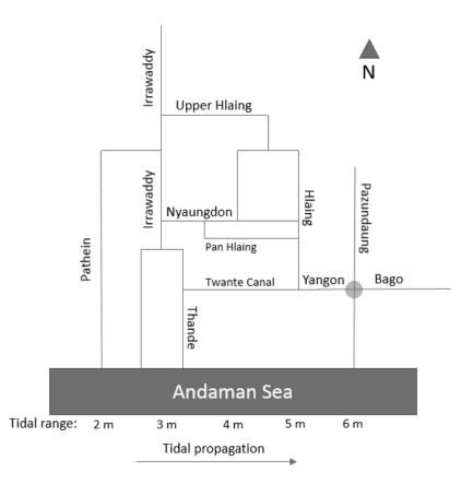
Figure 2.1: River network of the Irrawaddy Delta. The numbers show the increasing spring tidal range from West to East.
