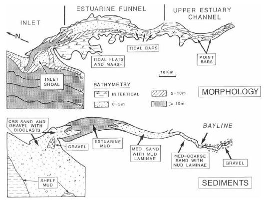
Figure 4.3: Morphologic and sediment conditions of the Gironde Estuary. Source: (Allen G., 1991).
