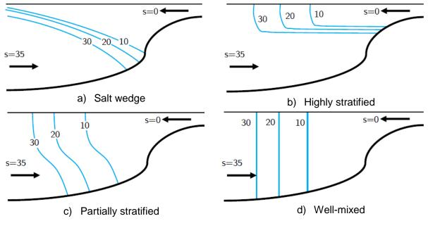
Figure 13.3: Types of stratification (Pritchard, 1967).
