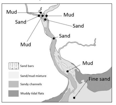
Figure 2.6: Sediment distribution in Yangon Estuary. Bullets represent sediment samples by JICA (2016).
