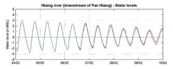
Figure 13.10: Simulated (blue) versus measured (red) water level at the confluence of the Pan Hlaing and Hliang River (station KIP) in the period of discharge measurements on the Pan Hlaing (February 5 2018)
