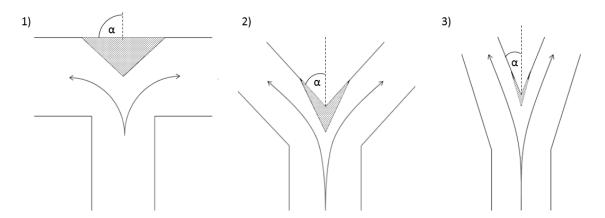
Figure 4.10: Schematisation of flow at a bifurcation with decreasing bifurcation angle from left to right: 1)  $\alpha$  = 90°, 2)  $\alpha$  = 45°, 3)  $\alpha$  = 20°. The grey area is referring to the sedimentation area in dive-up zone.
