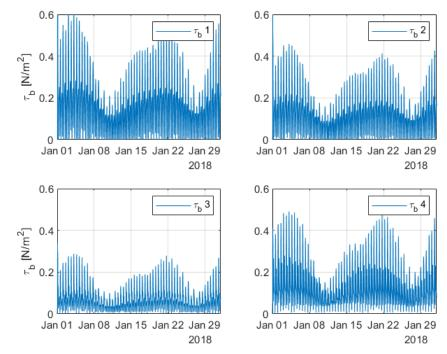
Figure 8.11: Bed shear stresses at point 1, 2, 3 and 4 in the enlarged Monkey Point Channel
