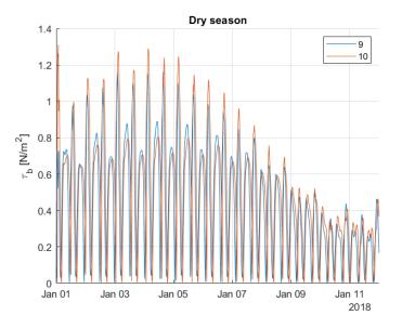
Figure 6.12: Bed shear stress on the northern shoal (9) and southern shoal (10) during the dry season. The maximum shear stress occur during spring tide and the minimum shear stresses occur during neap tide.
