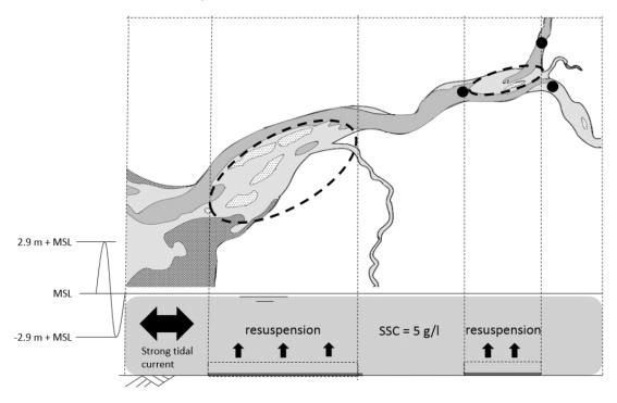
Figure 4.6: Conceptual diagram of resuspension of stationary and settled mud during spring tide. The black dots represent the locations where the SSC is measured.
