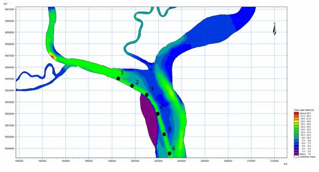
Figure 8.15: Bathymetry with dredged channel and the land reclamation. The numbered dots are the output locations used by the model
