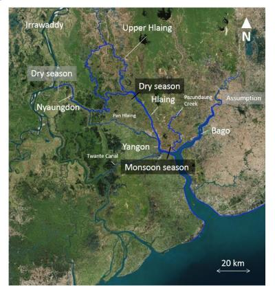
Figure 2.4: Tidal and salt intrusion. In black the salt intrusion limit during dry season and monsoon season. In grey the tidal intrusion limit in dry season. Tidal intrusion limit during monsoon is not known.
