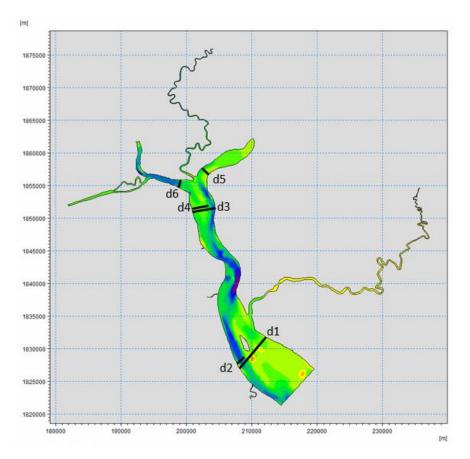
Figure 5.7: Cross-sections for calculating the discharges along the estuary
