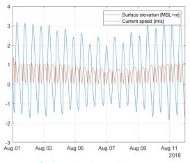
Figure 5.24: Surface elevation and current speed at location 3 during monsoon season
