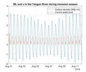
Figure 5.28: Surface elevation (WL) and current speed (u) in the Yangon River during monsoon season
