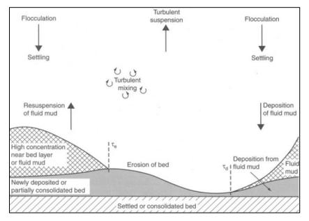
Figure 4.16: Cohesive sediment processes (Whitehouse, 2000)
