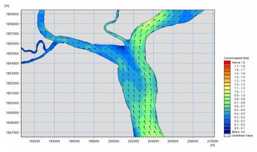
Figure 5.34: Current speed during neap flood in dry season
