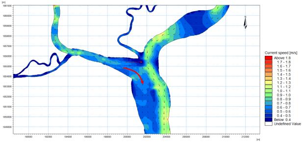
Figure 8.10: Flow velocities with direction during spring ebb in dry season. The large red arrow indicates the dominant flow and the smaller red arrow indicates the minor flow.
