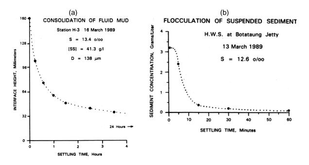
Figure 4.19: (a) Hindered settling of fluid mud taken from the Yangon River (Nelson, 2000). (b) Settling behaviour of suspended sediment sample taken from the Yangon River (Nelson, 2000).
