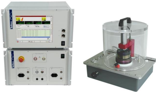
Fig.3. Left: The Tettex 2830 dielectric analyzer and right: Tettex 2914 test cell for solid insulants.
