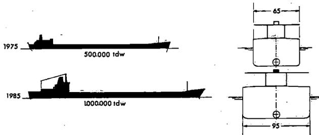
Fig. 2.10. Bridge-wings on ships with a beam larger than 65 m. It is clear that bridge-wings for looking alongside have to be replaced by other possibilities in the future.
