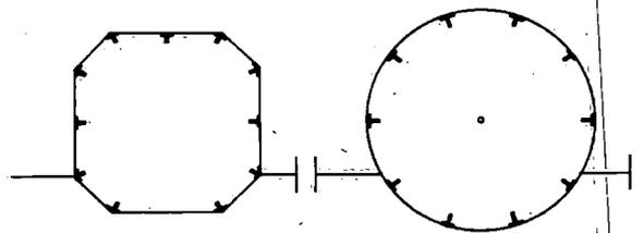
Fig. 2.8. A circular bridge, giving from the centre an optimum view outside. A bridge with straight sides (left) almost achieves this ideal groundplan.
