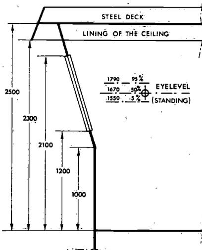
Fig. 2.6. Cross-section through a bulkhead of the bridge. The centre of the windows equals the average eye-level when standing.
