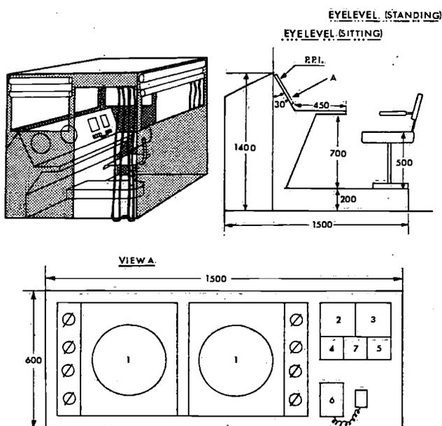
Fig. 2.18. Console inside the radar-cabin. The radar-cabin is to be used for longer observation periods, in which case the sitting position is favourable. Plotting can be done on the table. The table is illuminated in such a way that the intensity contrast between P.P.I. and table is acceptable (a standing position is also possible).
