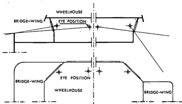
Fig. 2.1. Crosssection and groundplane of a bridge with and without view of the ship's sides, from the wheelhouse.
