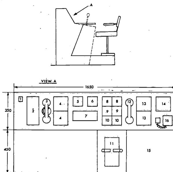
Fig. 2.14. The console for the O.O.W. on a twin-screw ship.
