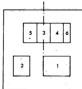
Fig. 2.4. Lay-out of the groundplan of the bridge. There is a gangway before the conning position, which makes obstruction of the helmsman's view possible.
