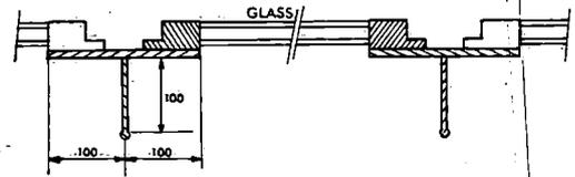
Fig. 2.7. Stiffeners between the windows with maximum dimensions.
