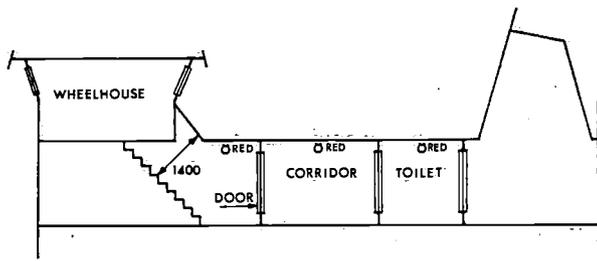
Fig. 2.9. Lighting of the gangway and staircase to the bridge. The door is important to prevent draught.
