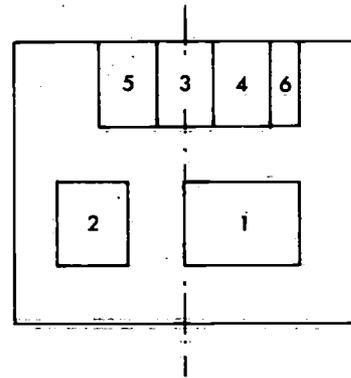
Fig. 2.3. Lay-out of the groundplan of the bridge according to 2.1. The conning position is situated against the front bulkhead.
