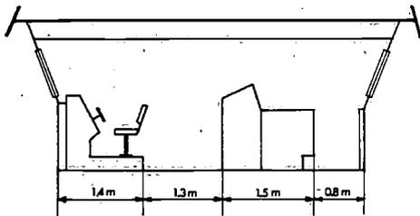
Fig. 2.5. Minimum depth of the bridge with the console against the front bulkhead.
