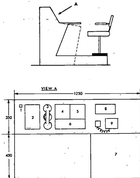
Fig. 2.15. The console of the O.O.W. with a qualified helmsman.
