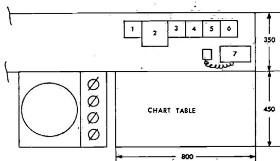
Fig. 2.20. View on the position of the pilot. For the side view see Fig. 2.16. If the dials are not readable from the pilot's chair, they are to be placed in the console in front of him.
