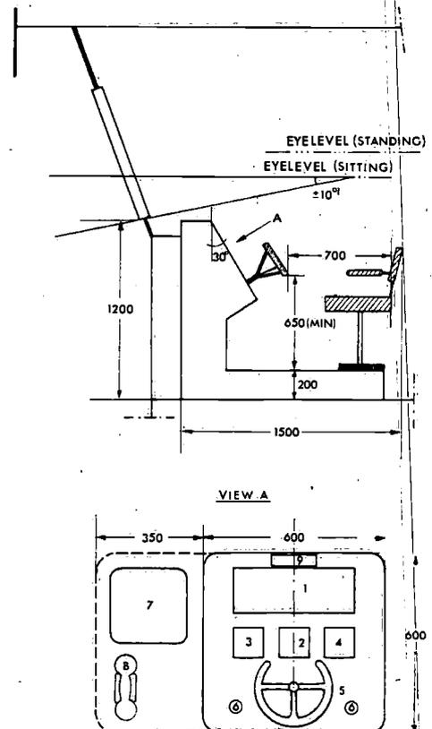
Fig. 2.12. The console for the helmsman.
