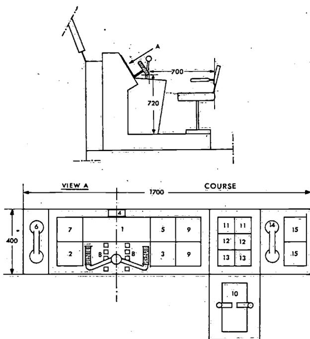
Fig. 2.13. The console for the helmsman on a twin-screw ship. For this case the helmsman should be highly qualified.
