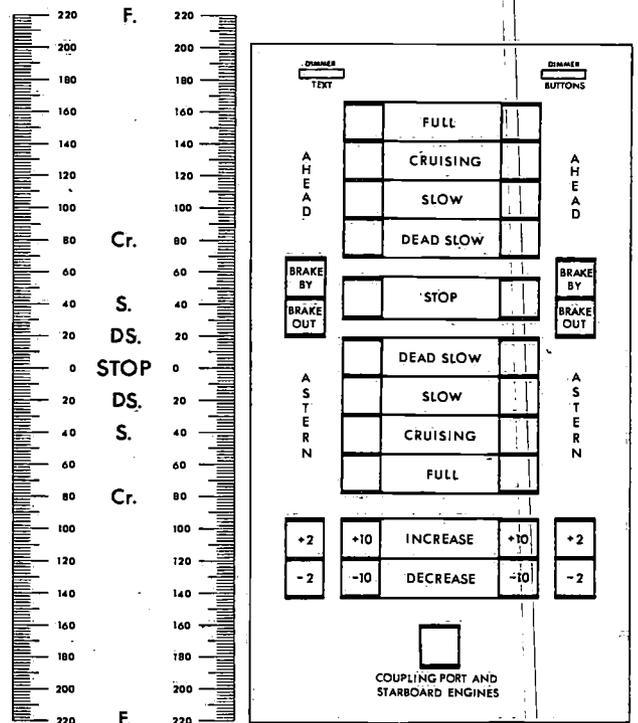
Fig. 2.22. Example of a push-button telegraph (right) and the scale of a conventional throttle telegraph, on a twin-screw ship. For the latter the desired revolutions of the shaft are adjusted with the throttle on the next points or between these. The same is the case with the push-button telegraph at night. In the condition ahead the r.p.m. can be adjusted with the push-button "increase" or "decrease". The other points equal those of the telegraph at left.
