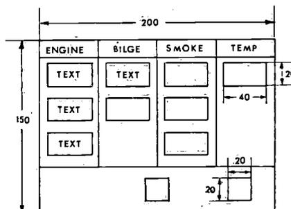
Fig. 2.21. Example of an alarm panel. Each group of alarms is represented by a rectangular warning light. The warning light starts flashing when there is an alarm. When the alarm has been accepted the light glows steadily and acoustic alarm ceases. The colour of all warning lights is red, the text shows the origin of the alarm. A test button and an acceptance button are also placed in the panel.
