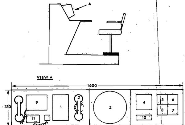
Fig. 2.16. The captain's console, which is an extended console with a radar to verify the near surroundings.
