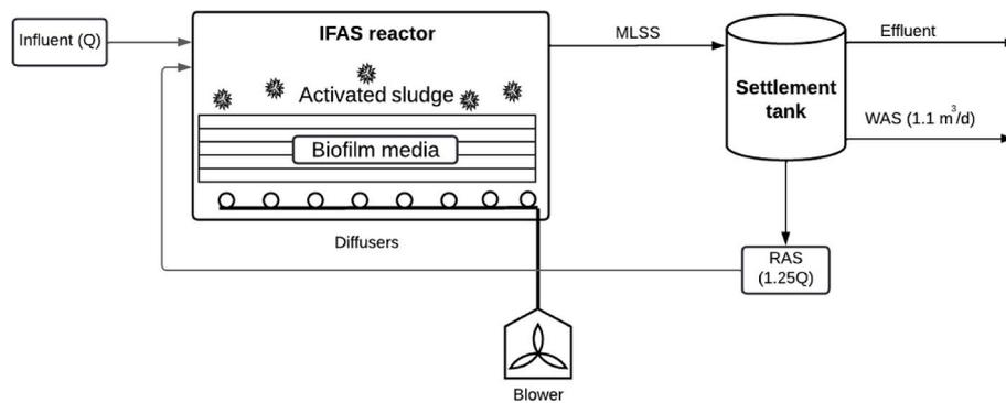
Fig. 1. Configuration of the package IFAS system.
