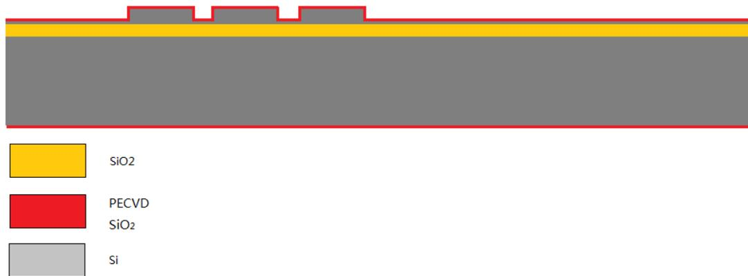
Figure 4-2 Cross section of the cantilever after PECVD SiO<sub>2</sub>.
