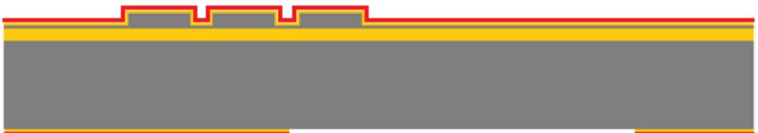
5. Because the substrate silicon is about 650µm thick, two etching steps are done, one using photoresist as mask and the second using silicon oxide. After 5 minutes DRIE, the photoresist is removed by acetone.
