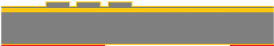
4. Coating front side with photoresist, then etch PECVD silicon dioxide by BHF1:7. As the etching rate of BHF1:7 is 1.2 nm/s, it takes at least 7 minutes. Then use DI water to wash it for 10 minutes.
