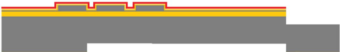
9. Continue with DRIE to etch from the backside step by step carefully, until the cantilever has been released. Then clean the photoresists remained on the chip front side.
