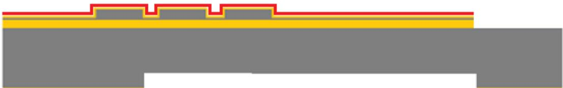
8. Since the etching rate for DRIE is  $5\mu\text{m}/\text{min}$ , and the total thickness of the beam totally is  $17\mu\text{m}$  ( $15\mu\text{m}$  silicon substrate adds  $2\mu\text{m}$  buried oxide), with about 3 and half minutes should be sufficient.
