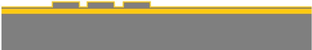
3. Define an open “window” in the oxide on the back side: coating with photoresist SR-3017, then baking the chip 1 minute at 95 C° after that exposure by contact lithography (see Figure 4-5), followed by baking at 115 C° 1 minute. Finally, develop the exposed photoresist by immersing the chip in MF-322 solution for 1 minute.
