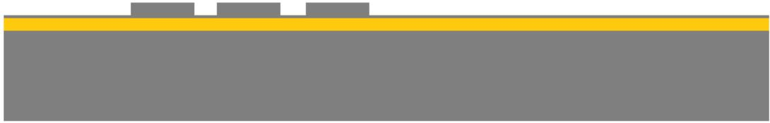
2. Deposit 500 nm of silicon dioxide by PECVD as a protection layer for the device layer. And on the back side as masking layer for the DRIE step.
