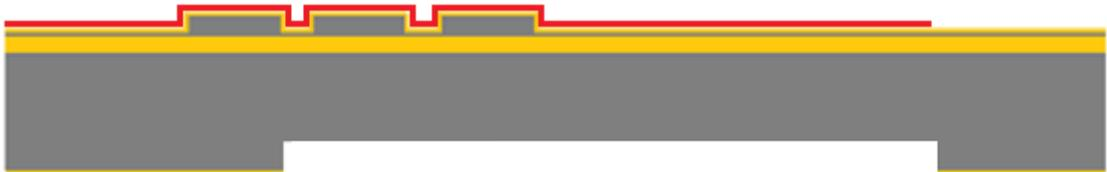
7. Open a window in front side by subsequent removal of oxide, silicon device layer and buried oxide. This is done by first an etch step in BHF1:7 solution for 7 minutes, followed by DRIE for 4 minutes and then again in BHF1:7 for at least 30 minutes followed by rinsing the chip 10 minutes with DI water.
