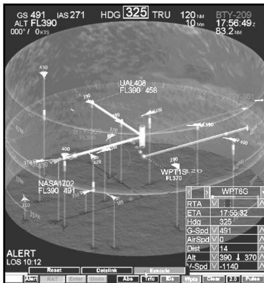
**Figure 2.22:** Three-dimensional cockpit situation display. This display presents traffic, weather, and terrain in a reconfigurable situation display. The pilot can select two-dimensional top and side views, as well as isometric and perspective views that can be panned, zoomed, and rotated. Figure taken from Battiste et al. [32].
