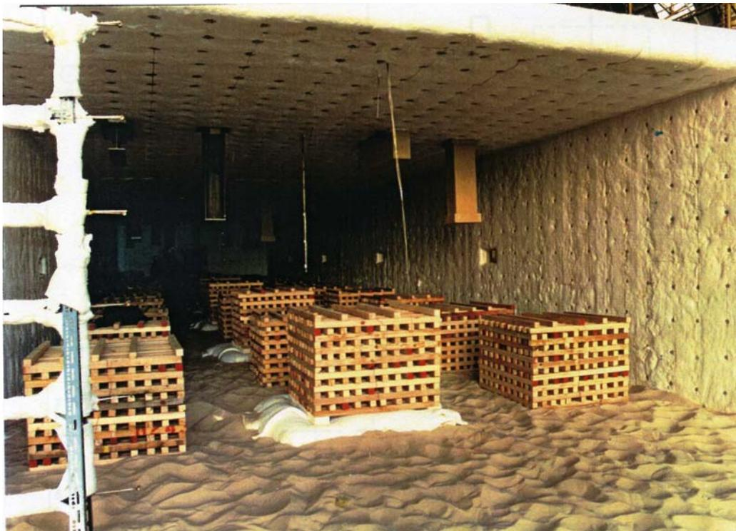
Figure 4: Construction of the wood cribs
