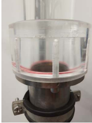
Figure 40: Plexiglas Flange with red O-ring
