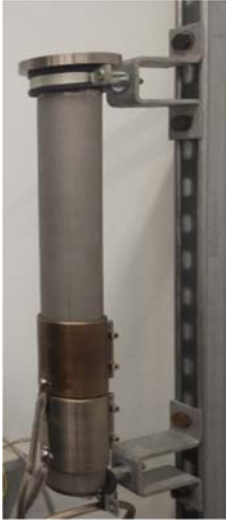
Figure 39: The Evaporator Tube
