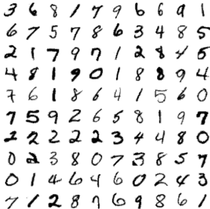
Figure 4.6: Sample from the MNIST database, showing the digits 0 to 9 in various handwriting styles. Each digit is an image of 28 by 28 pixels. From [21]
