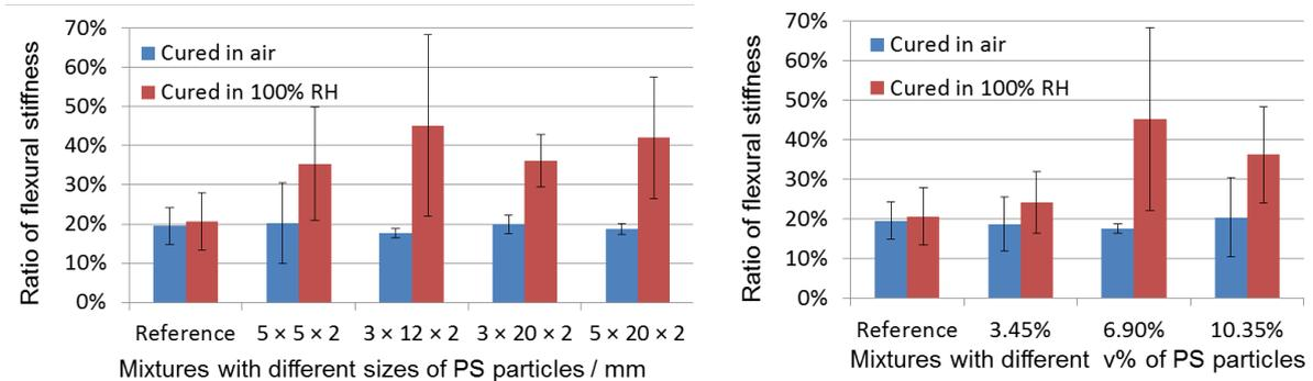
Figure 6: Ratio flexural stiffness ( $R_s$ ) of specimens
