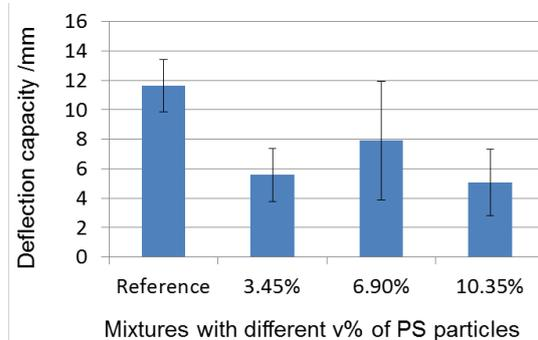
Figure 5: Flexural deflection capacity at 28 days
