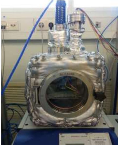
Figure 4.5: vacuum vessel used for testing the effects of vacuum on life-time of batteries
