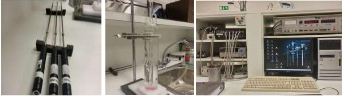
Fig. 4.1. a) IPRT sensors; b) Triple point of water cell; c) Readout set-up used to measure drift of NTCs, which includes AC resistance bridge and Keithley DMM.
