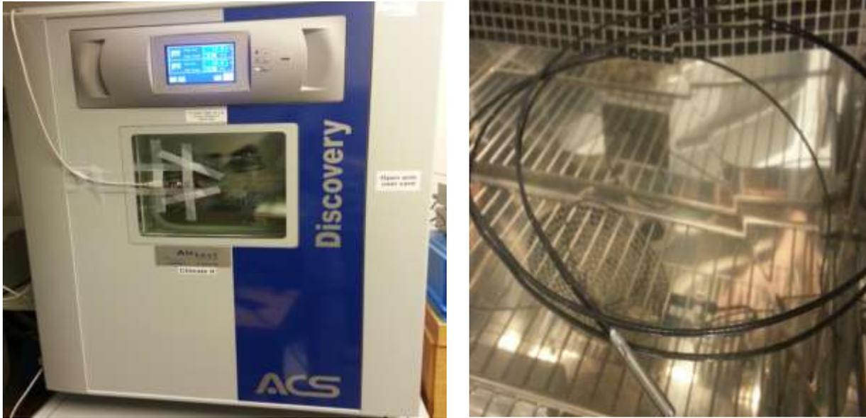
Fig 4.3 (a) Temperature chamber used to measure the transfer characteristics of the sensor (b) PT100 sensor
