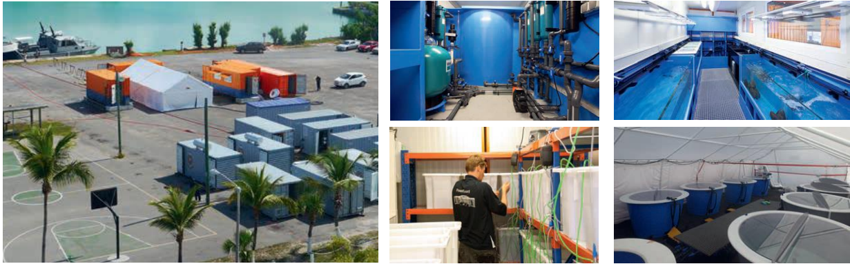
Figure 1. Left: ReefGuard facility (orange/blue containers and tent) operational in the Bahamas (August 2015); Middle-top: Filter container aimed at maintaining proper water quality; Middle-bottom: Wet laboratory designed to handle multiple smaller basins and to perform microscope inspections; Right-top: Aquarium laboratory designed to provide a high level of environmental control (container on the left in the top panel). Right-bottom: Patio area with a range of basins that can be used in various stages of the breeding process (from: Van Koningsveld et al. , 2017).
