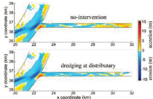
Figure 3. Erosion and accretion after two years of simulation without any intervention (top) and after dredging at the distributary river (bottom).
