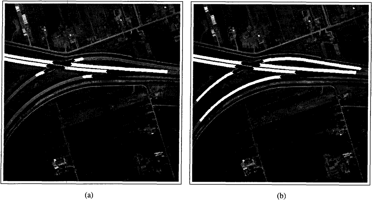
Figure 6.6: The new arcs, shown in white in (a), which are related to the new nodes, are identified during contextual reasoning. The final result of the interpretation is shown in (b).
